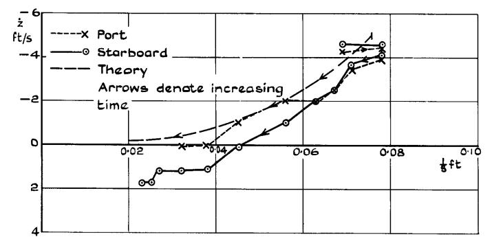
b Vertical velocity vs (half-separation)<sup>-1</sup>
