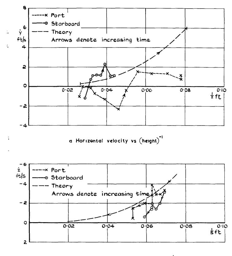
b Vertical velocity vs (half-separation)<sup>-1</sup>
