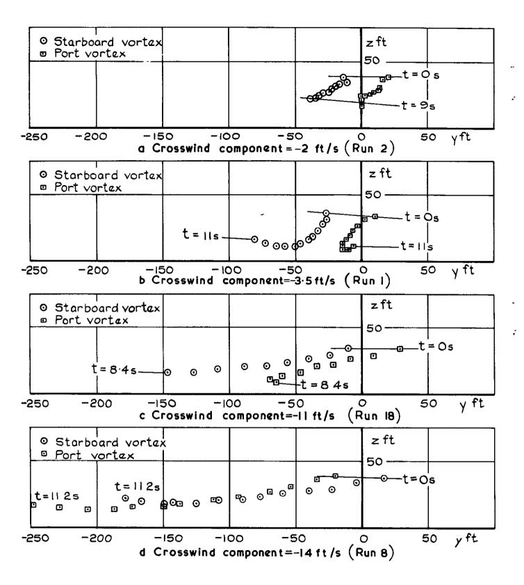
Fig 4a-d Measured vortex positions with different crosswind components
