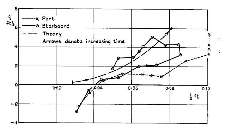
a Horizontal velocity vs (height)<sup>-1</sup>
