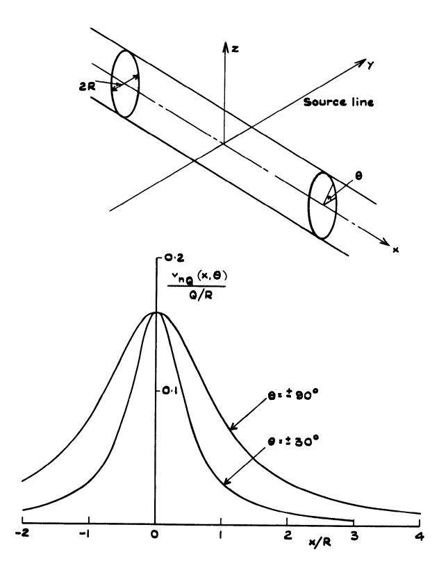
Fig.1 Normal velocity at the fuselage induced by a straight source line
