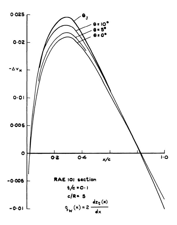
Fig.16 Streamwise velocity in the wing-body junction due to the source distribution on the fuselage
