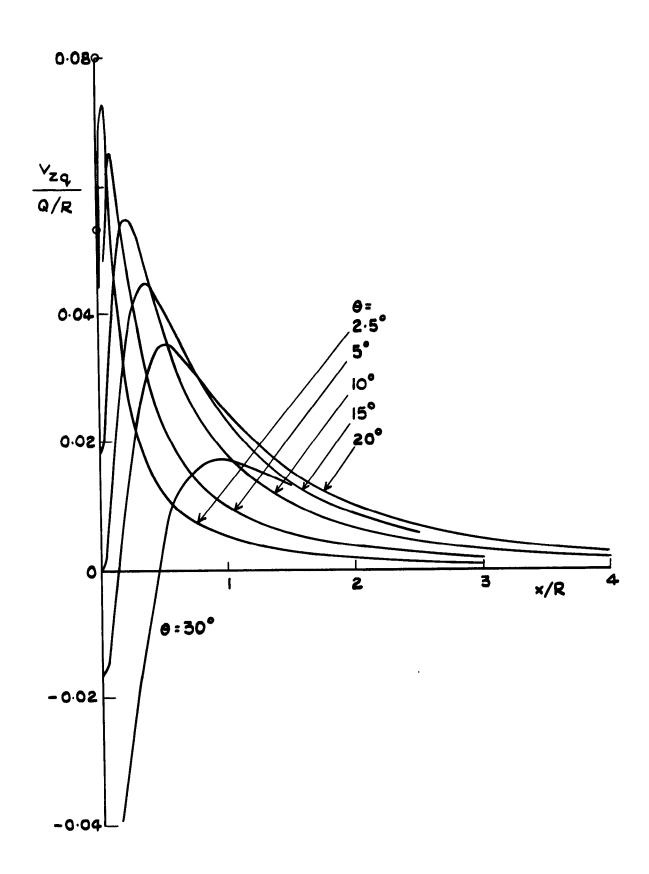
Fig. 12 vz-velocity component on the fuselage due to the source distribution on the fuselage
