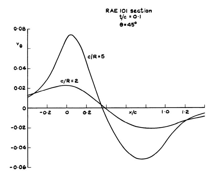
Fig. 20 Circumferential velocity component
