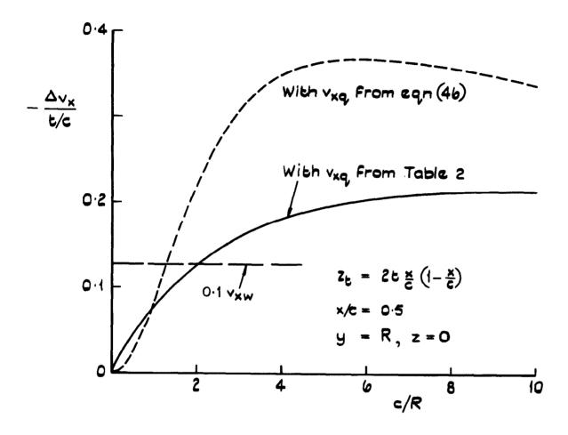
Fig.10 Velocity decrement at midchord of the wing-body junction for a wing with biconvex chordwise thickness distribution,
