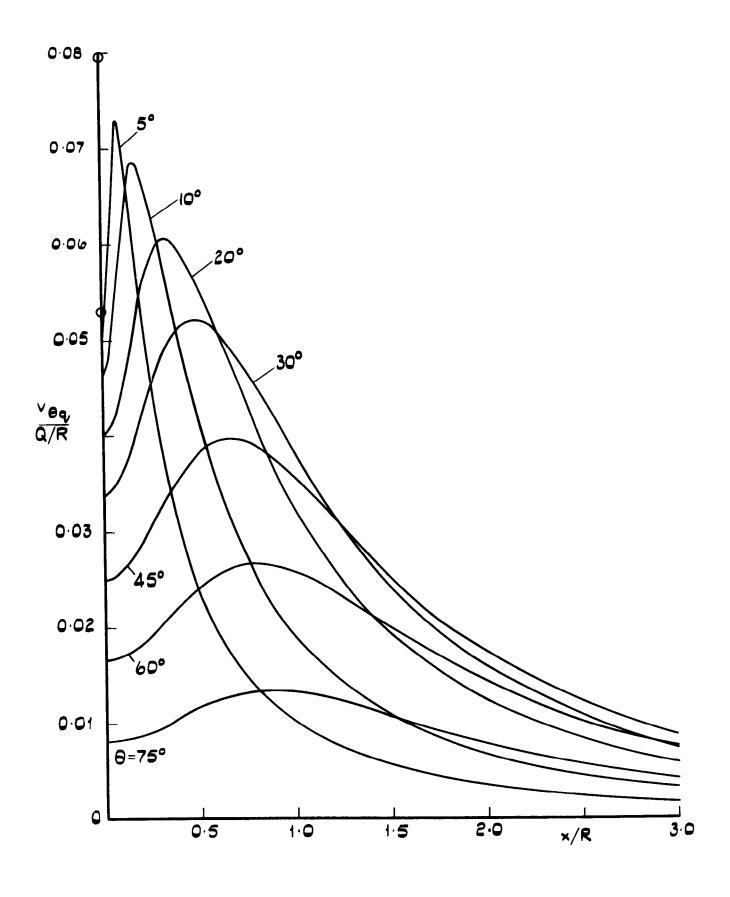
Fig.8 Circumferential velocity on the fuselage due to source distribution on the fuselage
