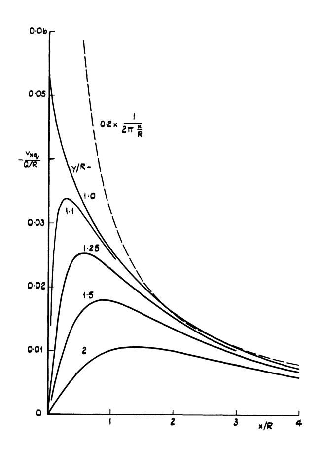
Fig.4 Additional streamwise velocity in the wing plane, z=0, induced by the source distribution on the fuselage
