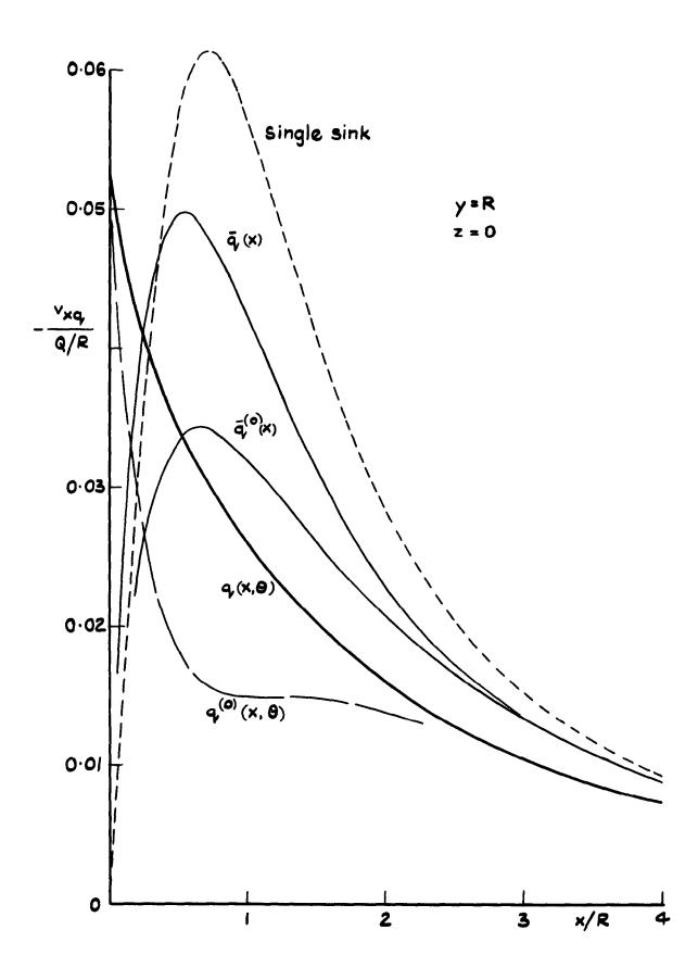
Fig. 5 Additional streamwise velocity in the wing-body junction
