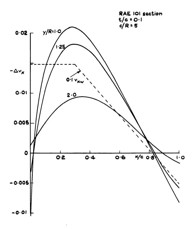
Fig. II Interference velocity in the plane of the wing
