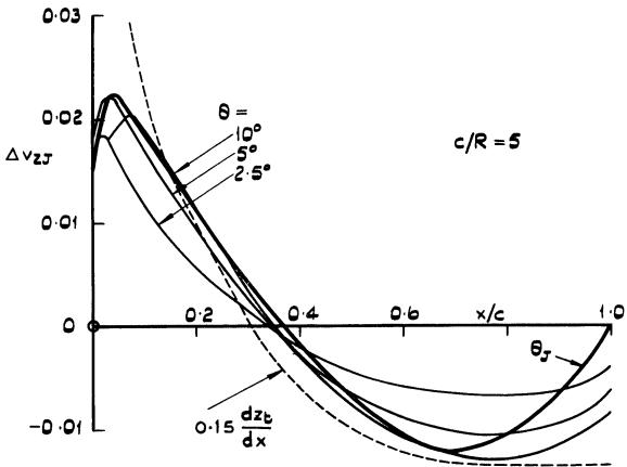
Fig.13  $v_Z$  - velocity component in the wing-body junction due to the source distribution on the fuselage
