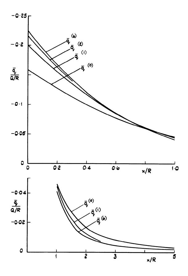
Fig.3 Average strength of source distribution on fuselage
