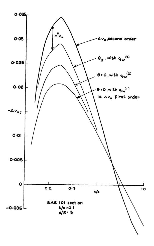
Fig. 17 Interference velocity in the wing-body junction
