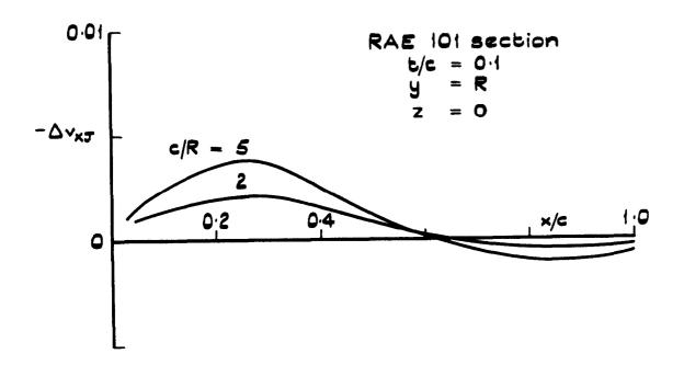
Fig.15 Change of interference velocity in the wing-body junction due to  $q_W^{(2)}(x) - q_W^{(1)}(x)$
