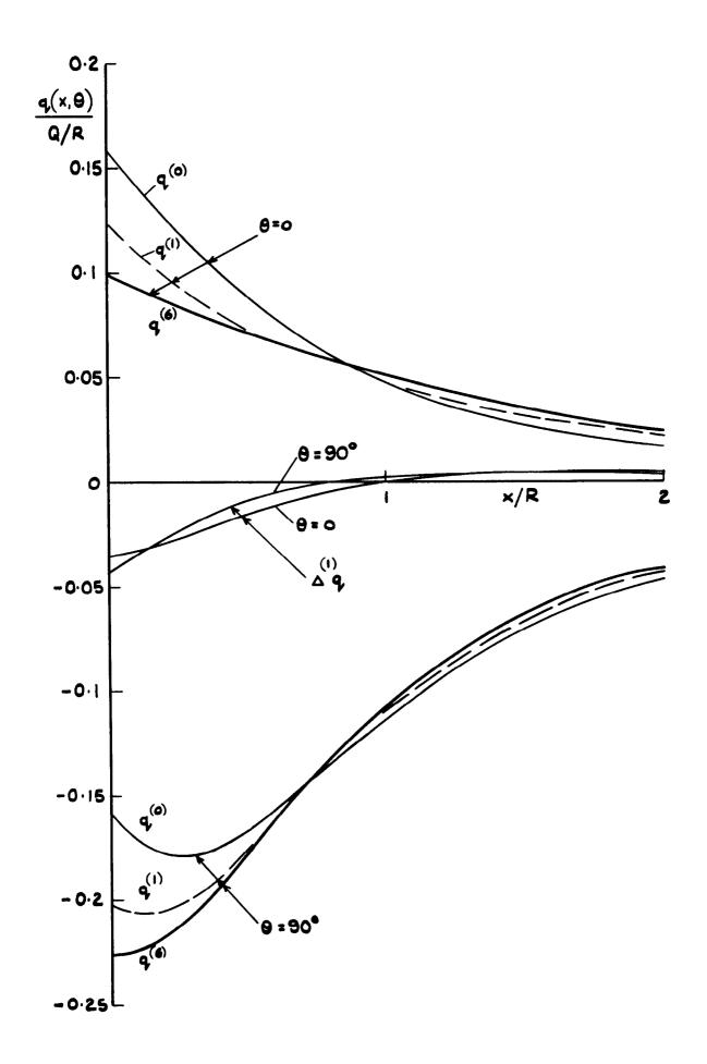
Fig. 2 Strength of source distribution on fuselage
