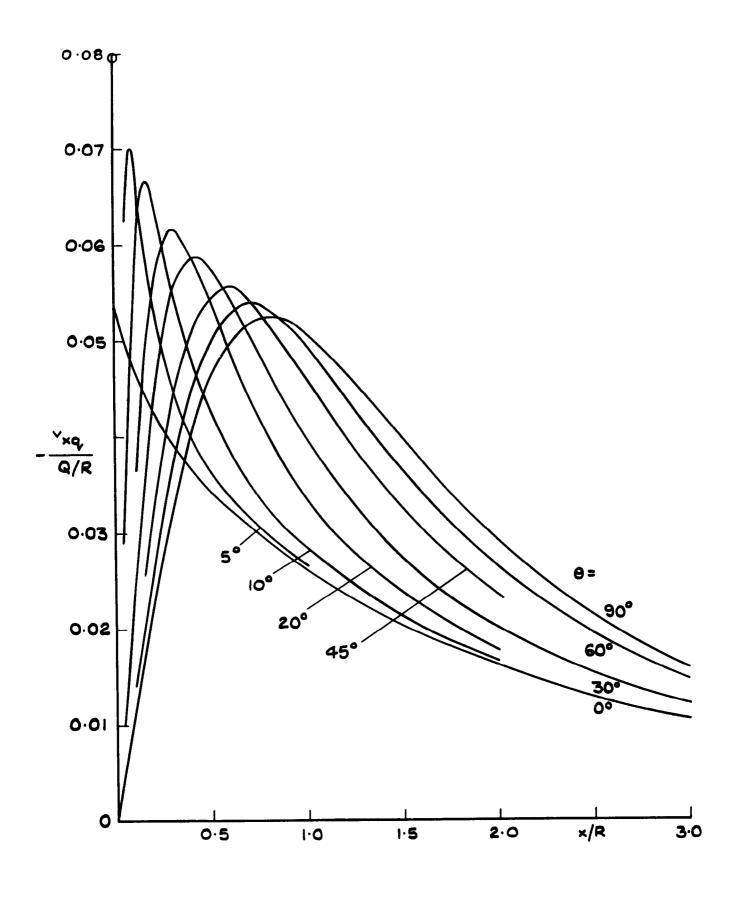
Fig. 6 Streamwise velocity on the fuselage due to source distribution on the fuselage
