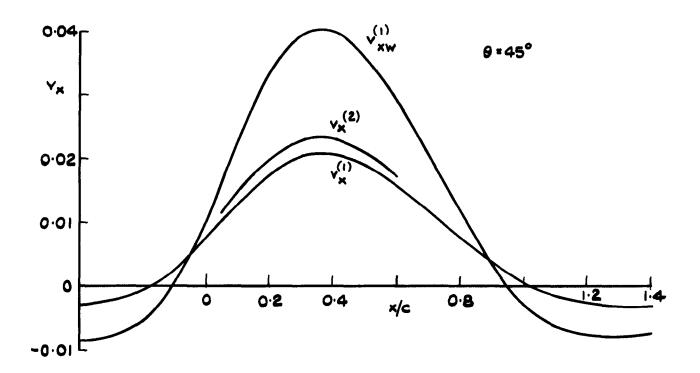
Fig. 18 Streamwise velocity component on the fuselage
