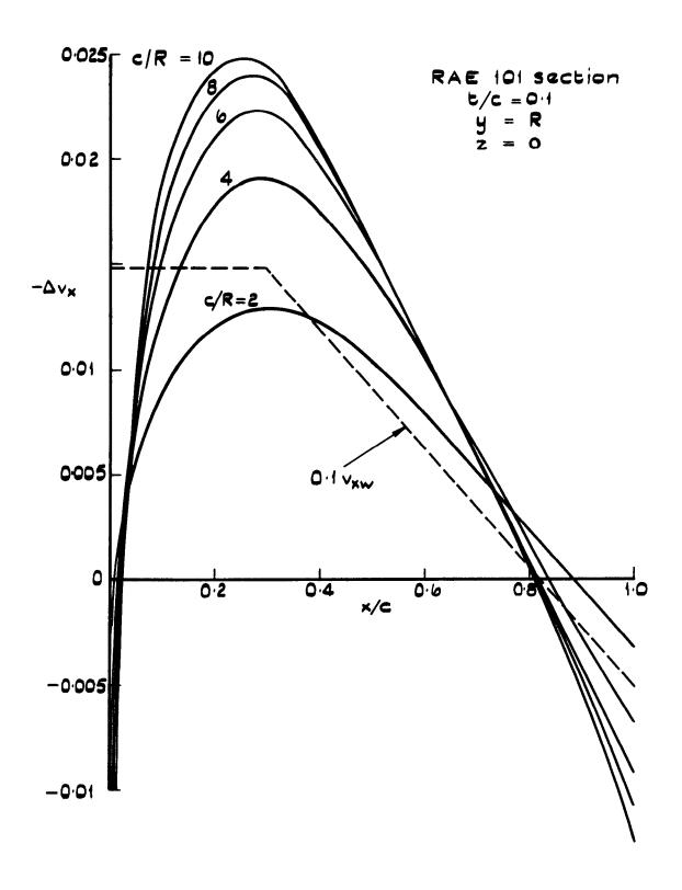
Fig.9 Interference velocity in the wing-body junction according to first-order theory
