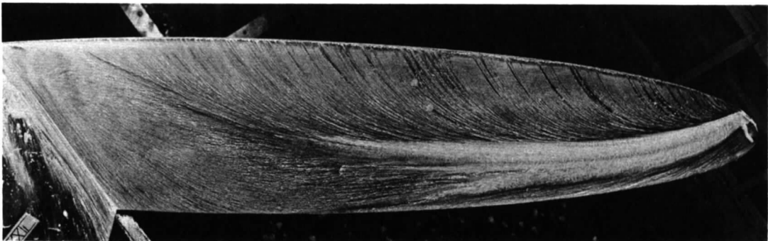
FIG. 24. Flow visualization at R_c = 1.02 \times 10^6 wire on.
