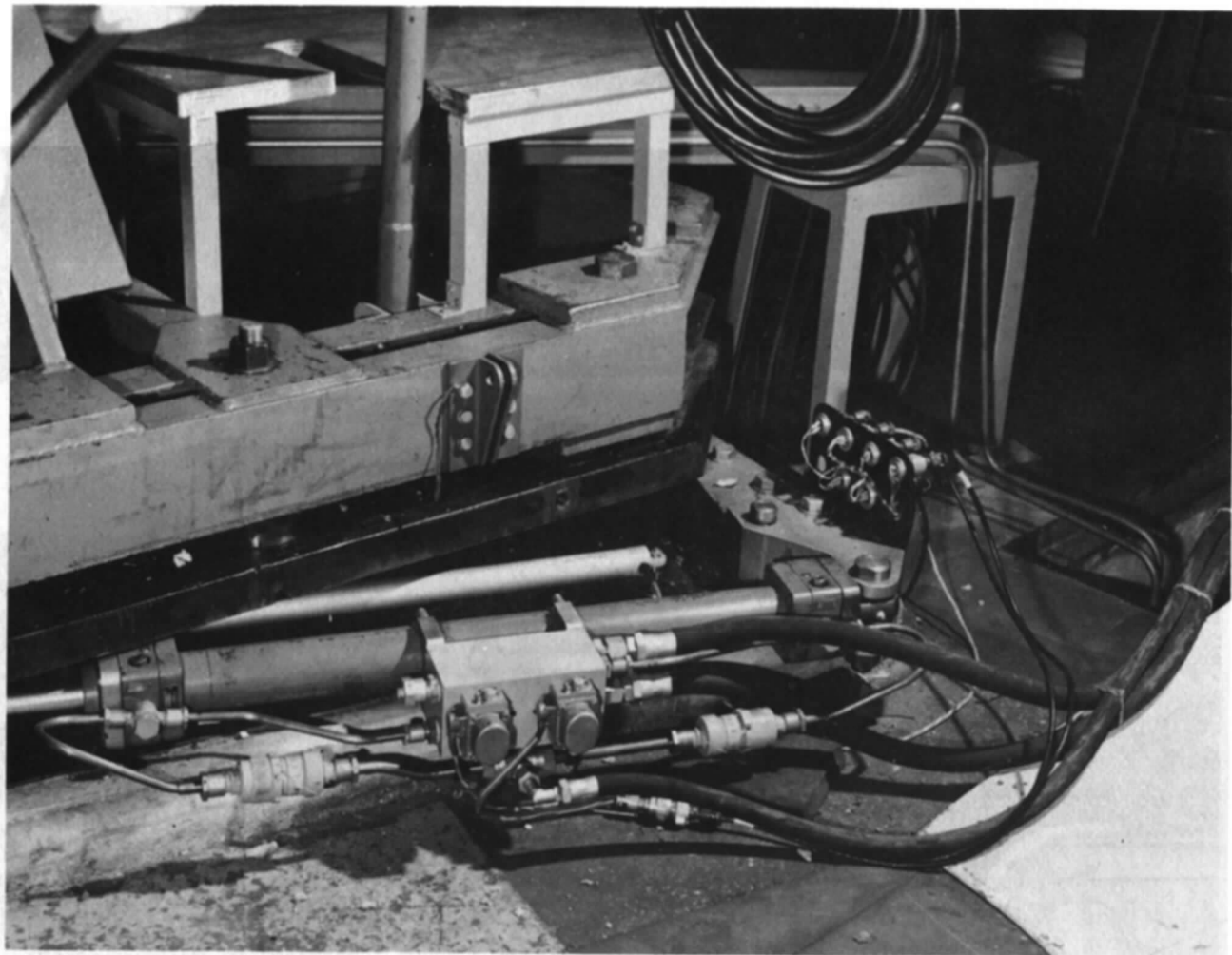
FIG. 8. Yaw freedom hydraulic servo drive assembly.
