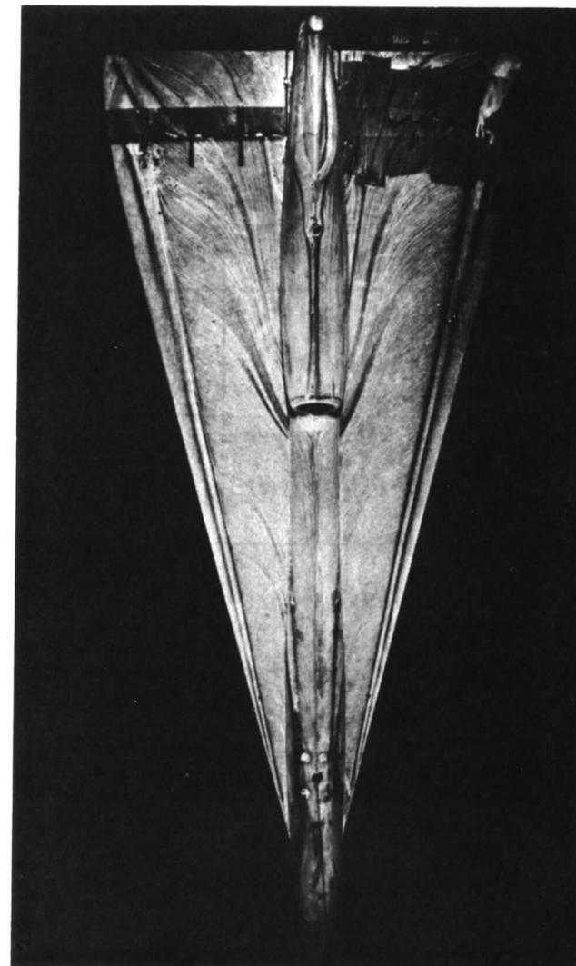
FIG. 8. Surface flow on  $\frac{1}{8}$  scale model with elevons undeflected (a)  $\alpha = 10^\circ$ ; (b)  $\alpha = 20^\circ$ , starboard hinge-gap unsealed.
