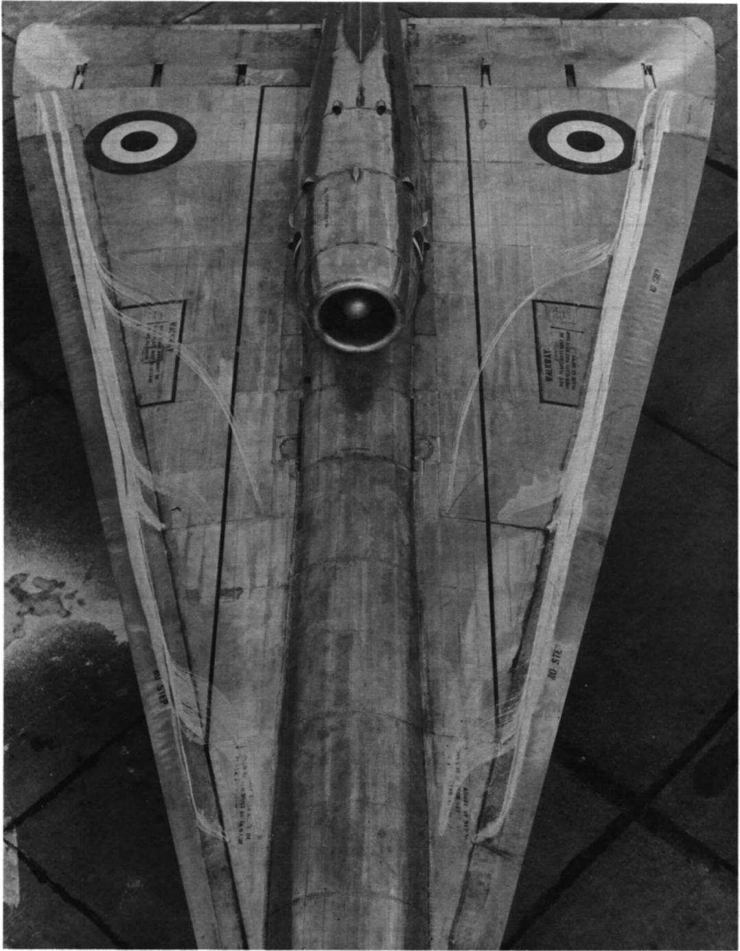
Incidence  $\sim 17.5^\circ$  Sideslip  $\sim -4^\circ$
