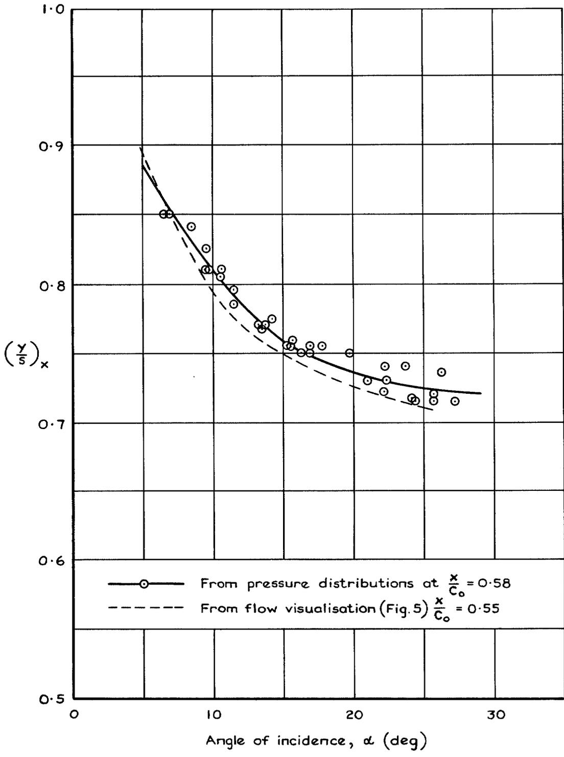
FIG. 7. Comparison of peak suction positions derived from pressure distributions with those deduced from flow visualisation.
