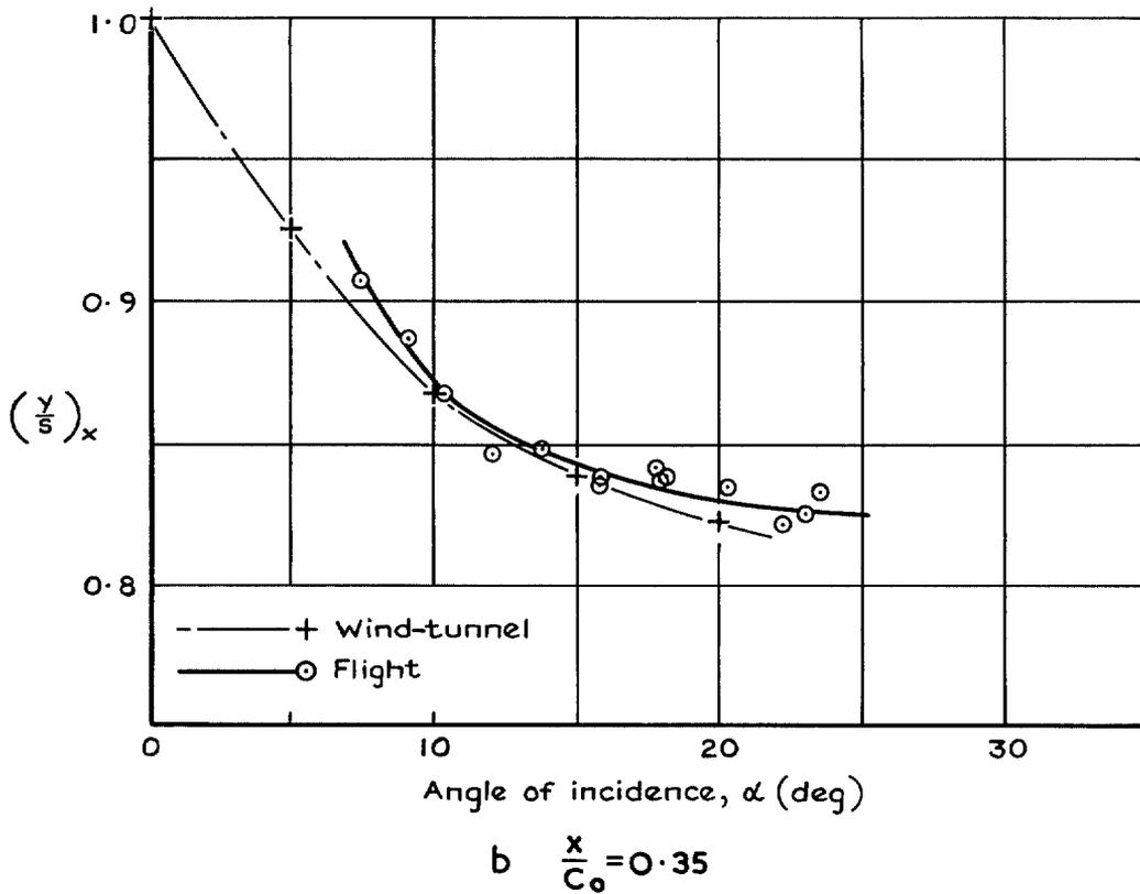
FIG. 9a and b. Comparison of secondary separation positions observed in flight and in wind-tunnel.
