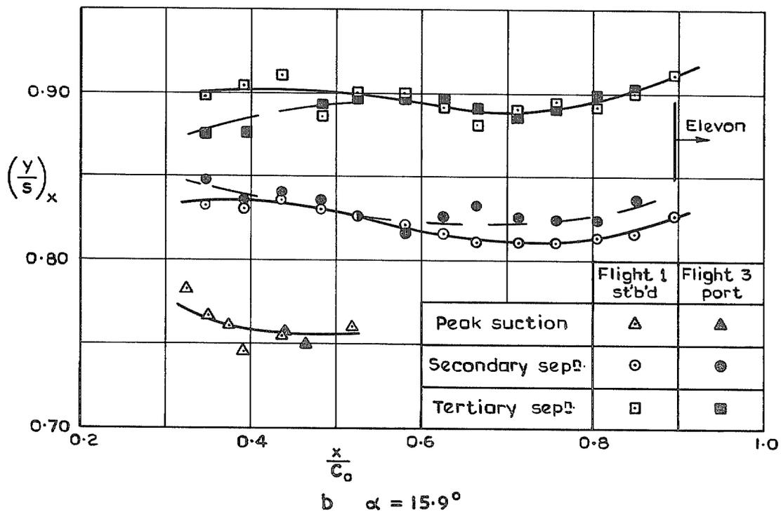
FIG. 4a and b. Plan position of typical surface flow features.
