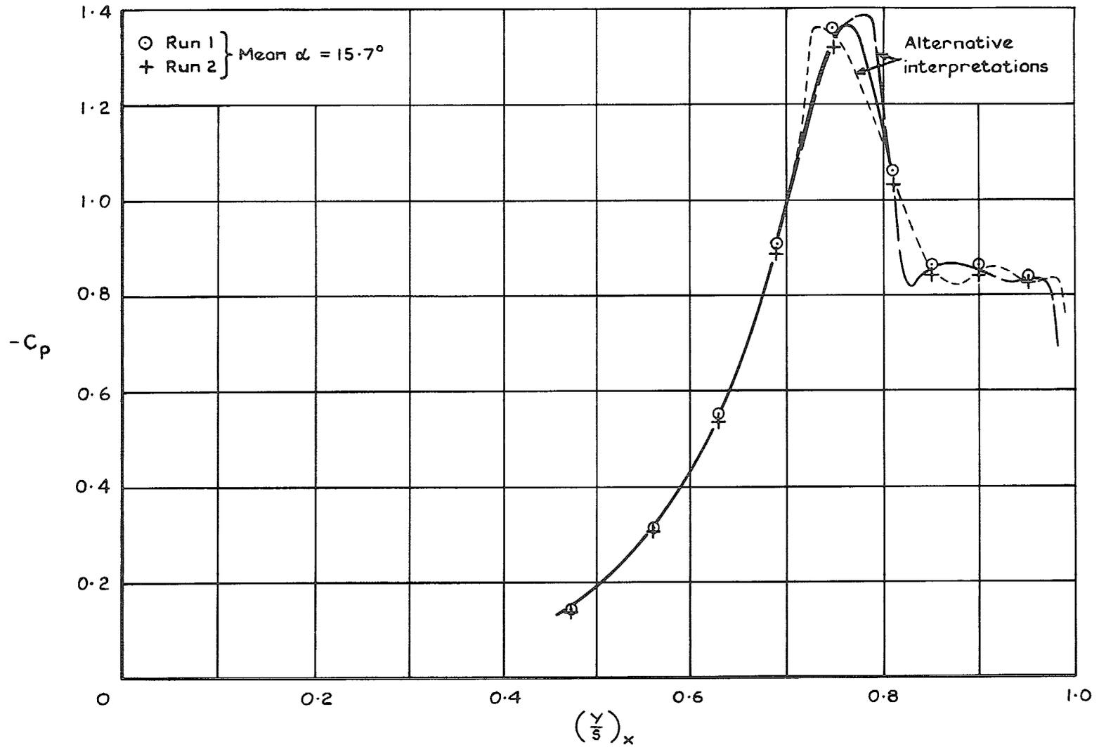
FIG. 6. Typical spanwise variation of pressure coefficient at  $x/C_0 = 0.58$ .
