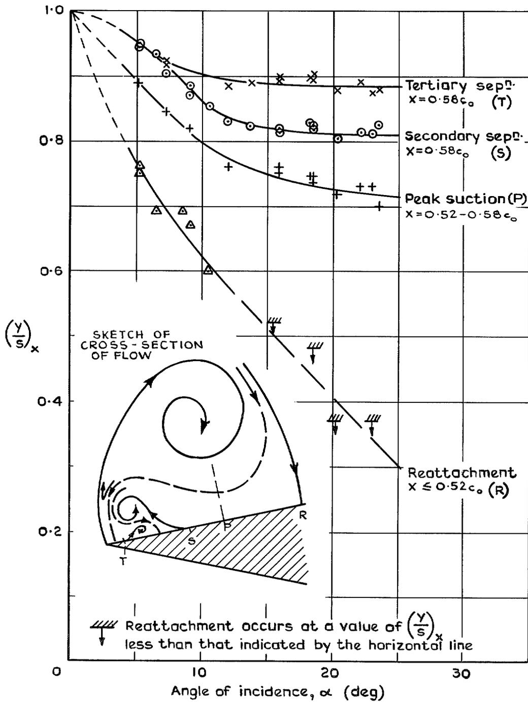
FIG. 5. Variation with incidence of spanwise position of major flow features.
