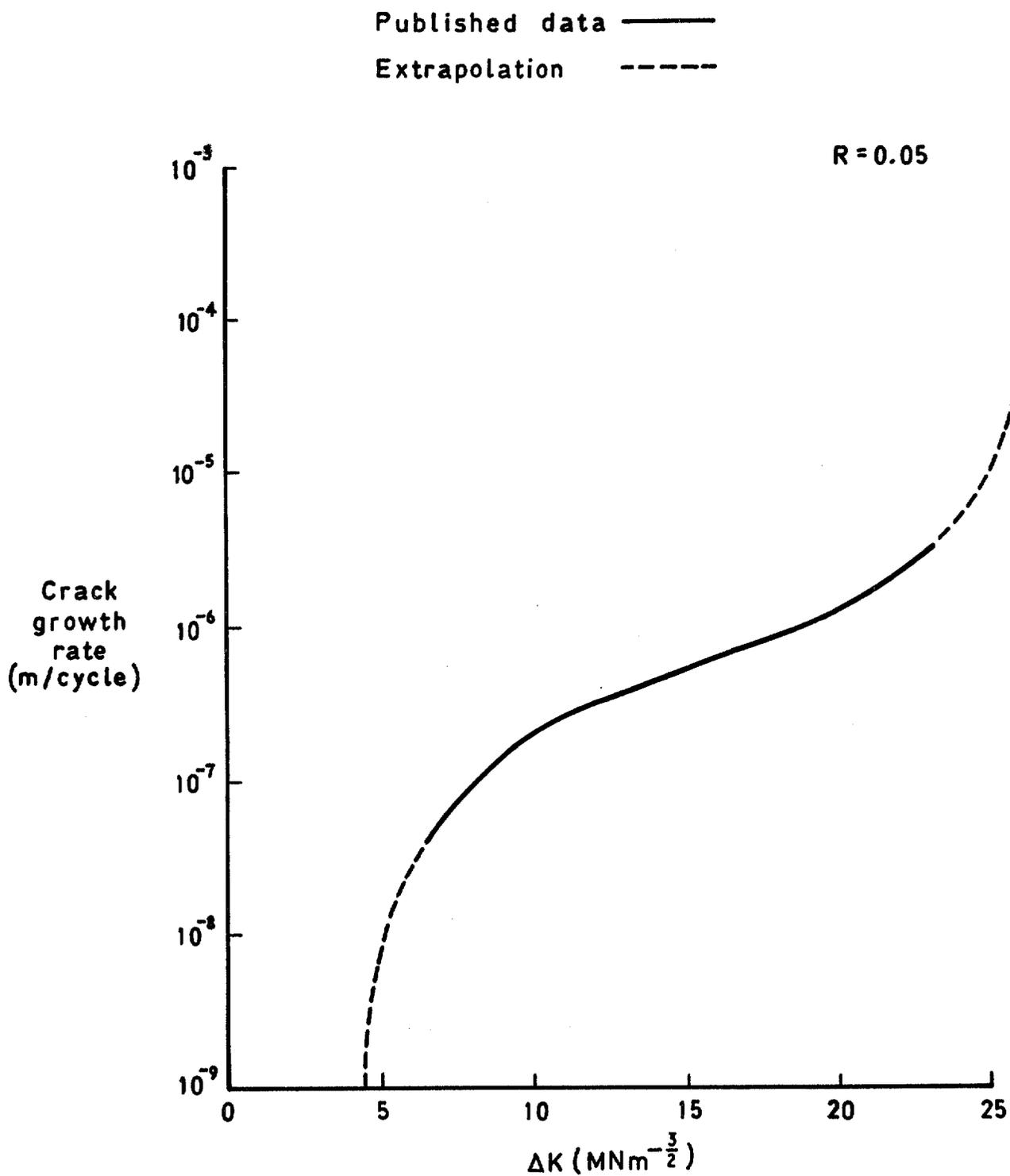
Fig 3 Extrapolation of da/dN vs  $\Delta K$  curve for DTD 5050
