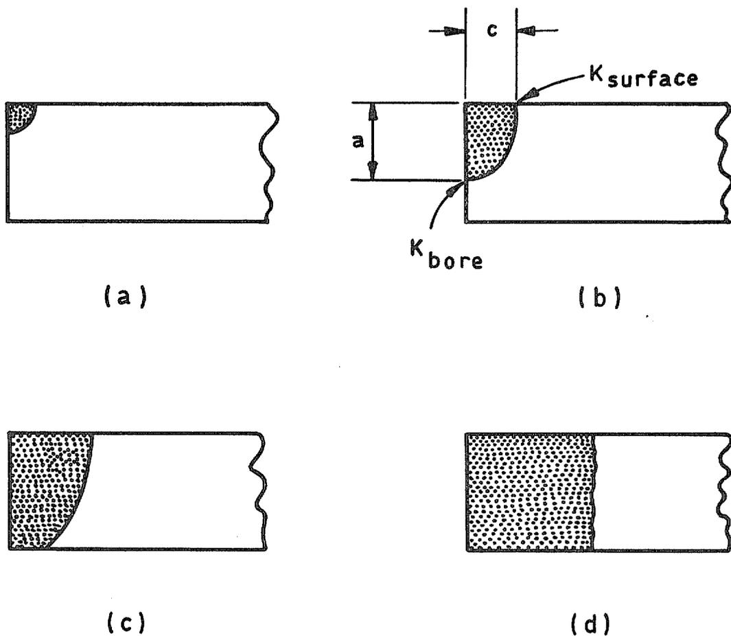
a Length of crack down the bore of the hole
