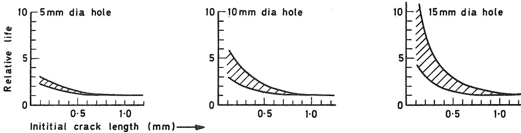
b Effect of initial crack length on life
