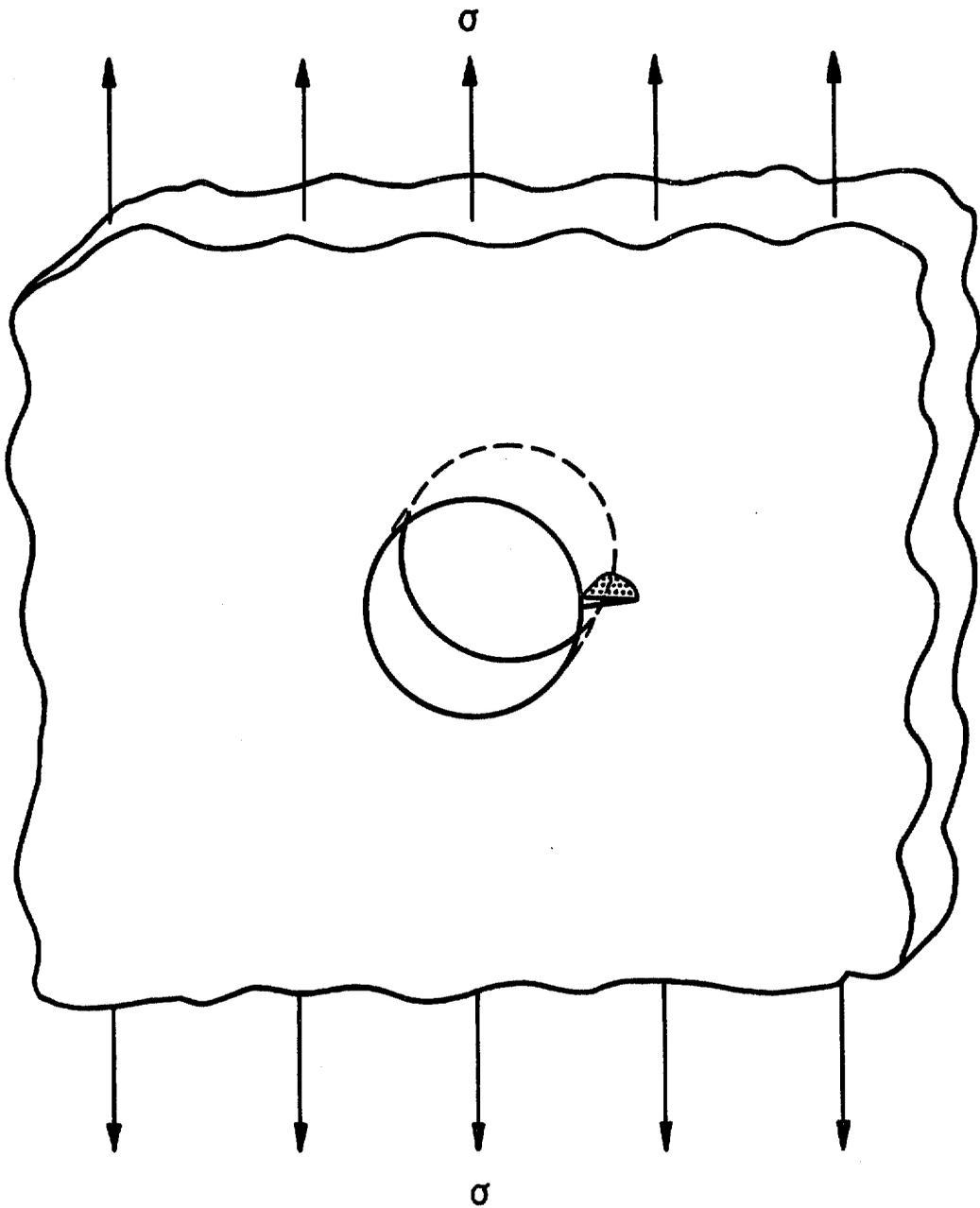
Fig 1 Corner-cracked hole in plate under uniaxial loading
