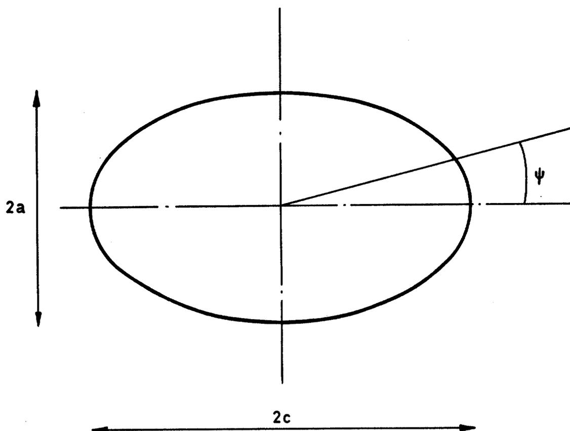
Fig 9 Notation for stress intensity factor of an embedded ellipse
