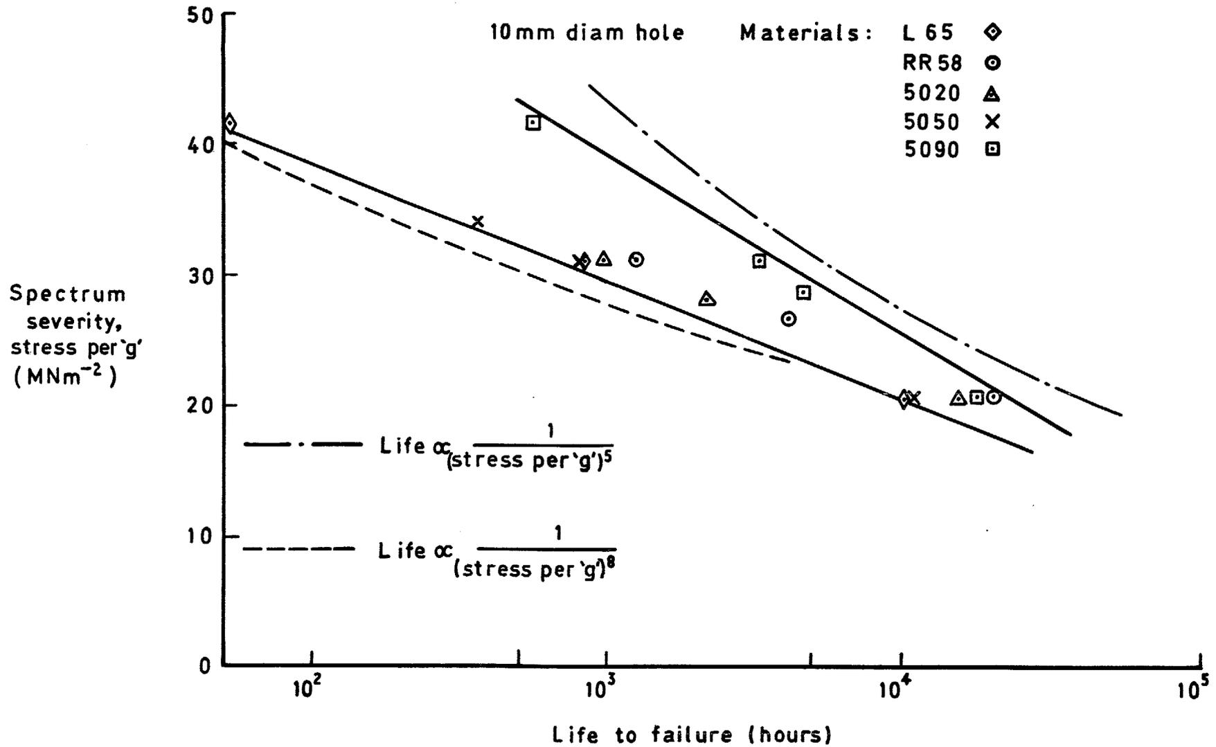
Fig 7 Effect of spectrum severity on endurance (1.25mm initial crack)
