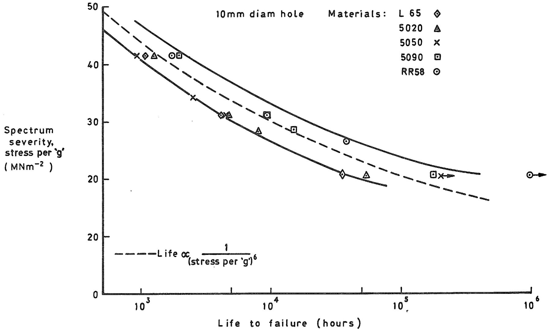
Fig 6 Effect of spectrum severity on endurance (0.125mm initial crack)
