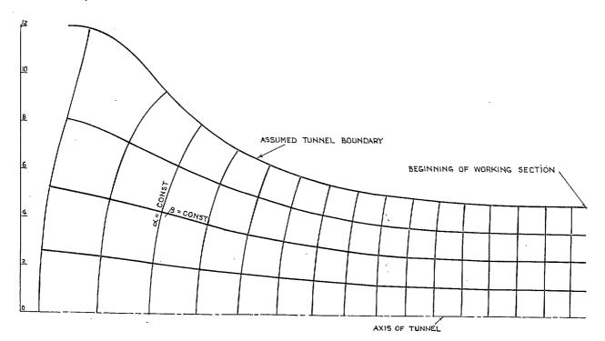
FIG. 1. Two dimensional network of stream and equipotential lines used as grid for the case of axial symmetry.
