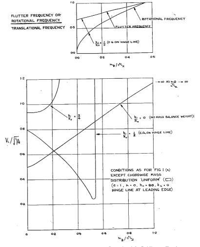
FIG. 1(b).—Variation of Flutter Speed with Stiffness Ratio and Various Degrees of Mass Balance.
