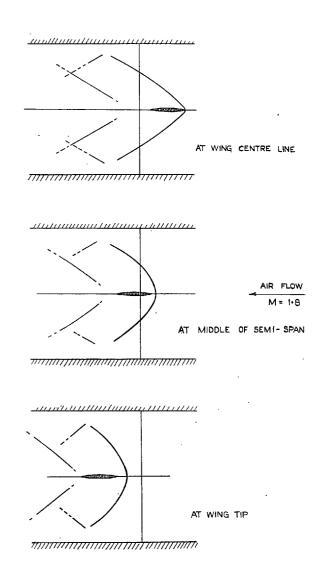
FIG. 10. Shock-wave configuration about a 50 deg. swept-back wing, M = 1.8. Incidence = 0 deg. Sections in line of flight, perpendicular to the plane of the wing.
