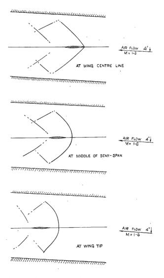
FIG. 8. Shock-wave configuration about a 50 deg swept-back wing, M = 1.6. Incidence = 4 deg. Sections in line of flight, perpendicular to the plane of the wing.
