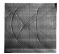
PHOTOGRAPH OF THE SHOCKWAVES IN A PLANE 0.66 INS. BELOW THE WING M= 1.4, INCIDENCE = 4°
