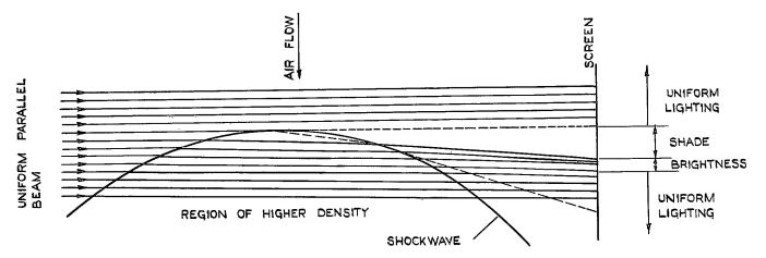
FIG. 3. Diagram illustrating the passage of a parallel beam of light through a curved shock-wave.
