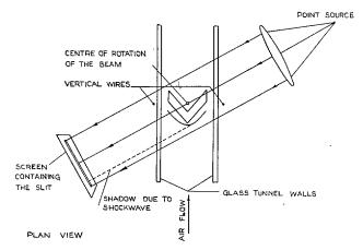
FIG. 2. The three-dimensional shock-wave recorder shown diagrammatically.
