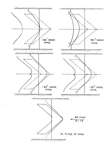
FIG. 9. Shock-wave configuration about a 50 deg sweptback wing, M = 1.8. Incidence = 0 deg. Sections parallel to the plane of the wing.
