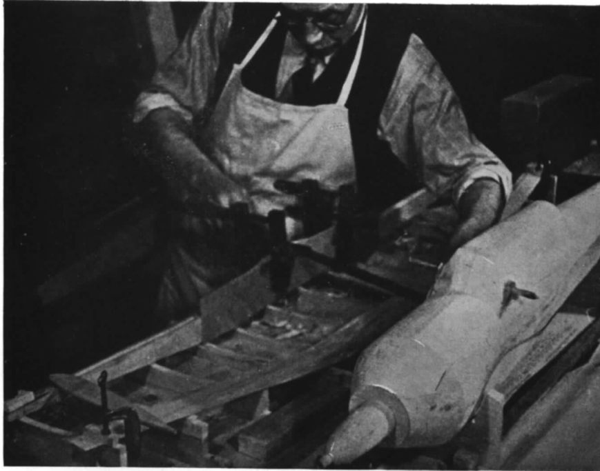
FIG. 7. A dynamic model under construction.
