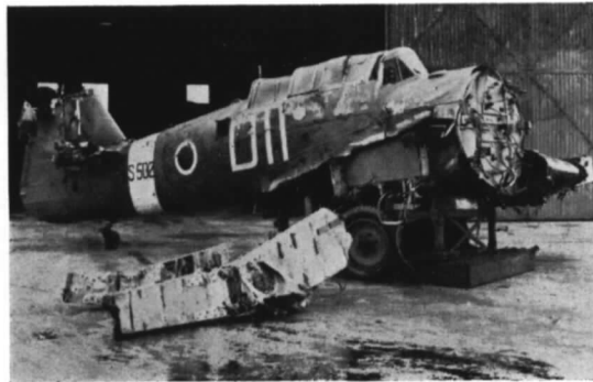
FIG. 19. Damage sustained by Martinet in ditching.
