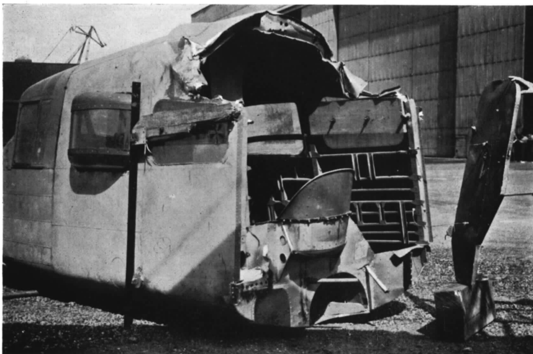
Damage sustained by dropping.
