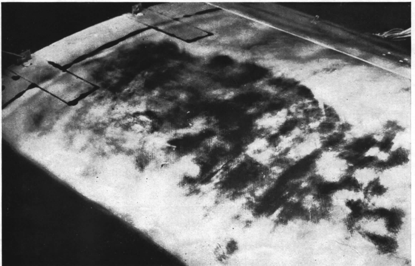
FIG. 4. Striations in laminar boundary layer. \Gamma = 50 deg, V = 160 ft/sec, transition at 55 per cent chord.
