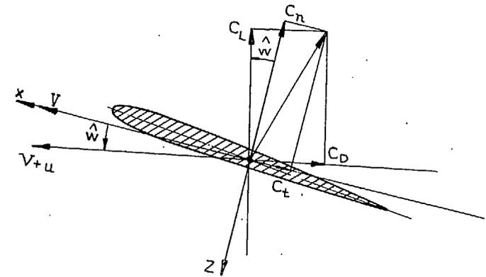
FIG. 5. 'Normal' and 'tangential' force coefficients  $C_n, C_t$ .
