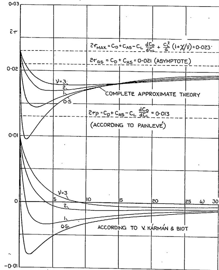
FIG. 7b. Phugoid damping factor for varying  $\omega$  and  $\nu$ , at low incidence.  $C_L = 0.2$ ,  $C_D = 0.014$ ,  $C_{AS} = 0.007$ ,  $a = 4$ ,  $\chi = 0$ .
