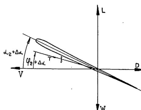
FIG. 3b. Aircraft at modified speed and incidence.
