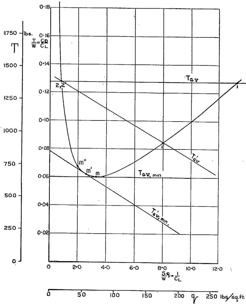
FIG. 1. Curves of thrust required and available for determining performance illustrating Painlevé's stability criterion.  $C_{D0} = 0.009, s = 0.1$ .
