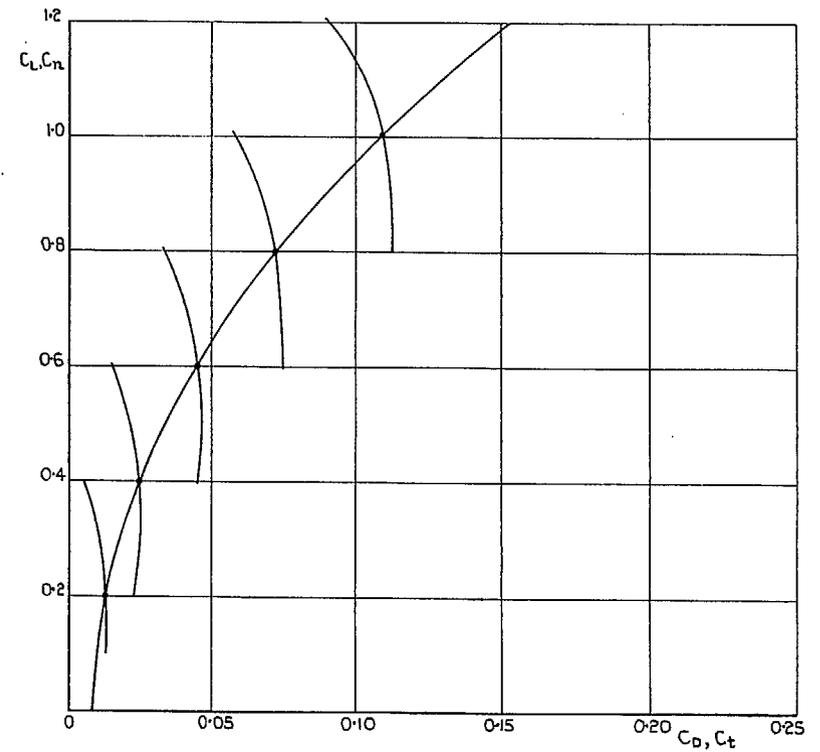
FIG. 6. Usual  $C_D$  vs.  $C_L$  polar curve and  $C_t$  vs.  $C_n$  polar curves.
