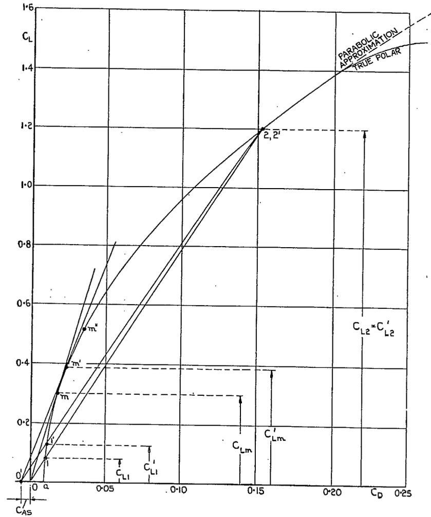
FIG. 2. Polar curve for determining performance, illustrating Painlevé's stability criterion.  $C_{D0} = 0.009, s = 0.1$ .
