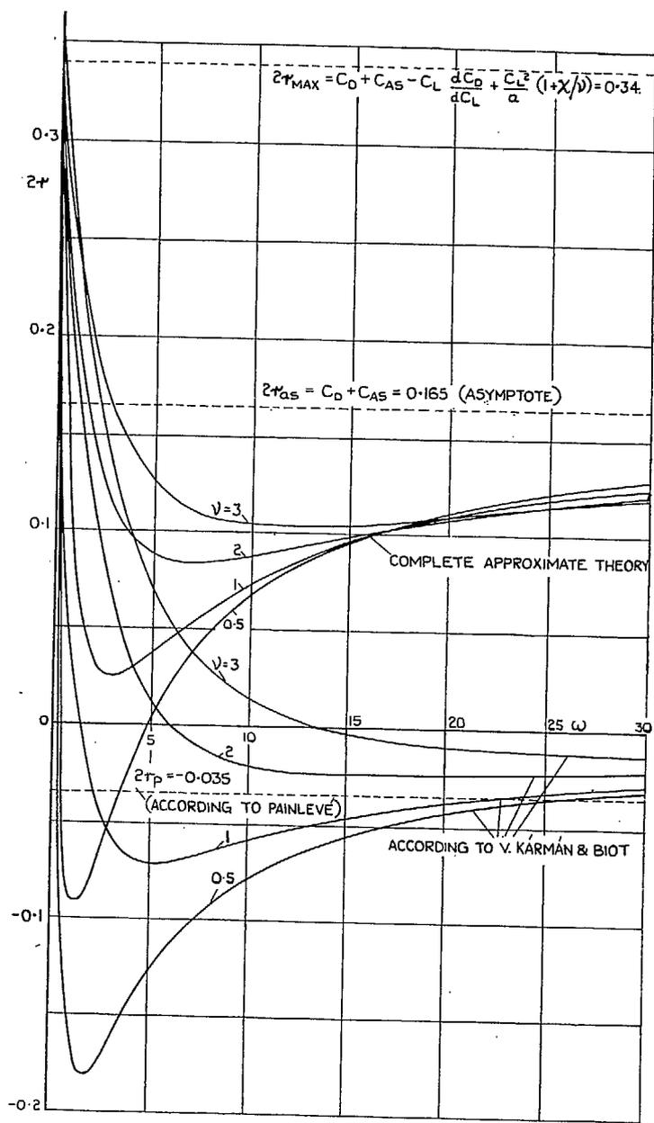
FIG. 7c. Phugoid damping factor for varying  $\omega$  and  $\nu$ , at high incidence.  $C_L = 1$ ,  $C_D = 0.11$ ,  $C_{AS} = 0.055$ ,  $a = 4$ ,  $\chi/\nu = 0.5$ .
