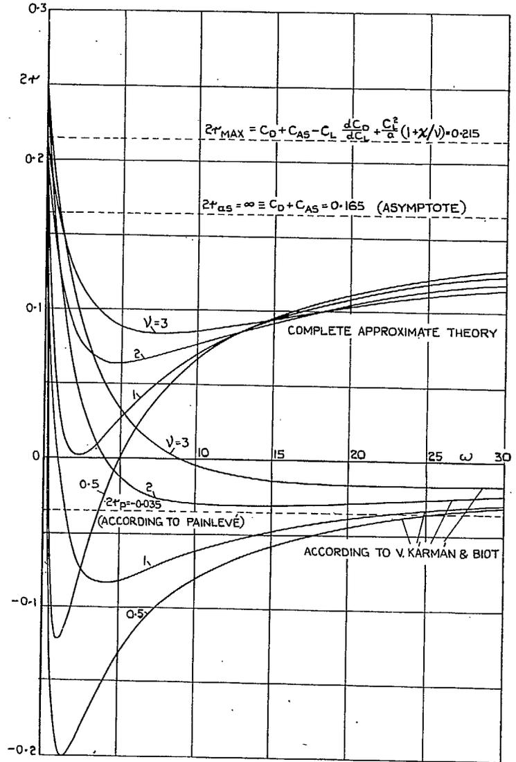
FIG. 7d. Phugoid damping factor for varying  $\omega$  and  $\nu$ , at high incidence.  $C_L = 1$ ,  $C_D = 0.11$ ,  $C_{AS} = 0.055$ ,  $a = 4$ ,  $\chi = 0$ .
