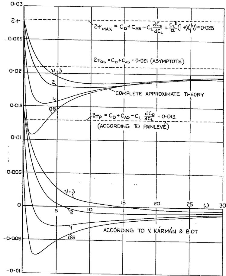
FIG. 7a. Phugoid damping factor for varying  $\omega$  and  $\nu$ , at low incidence.  $C_L = 0.2$ ,  $C_D = 0.014$ ,  $C_{AS} = 0.007$ ,  $a = 4$ ,  $\chi/\nu = 0.5$ .
