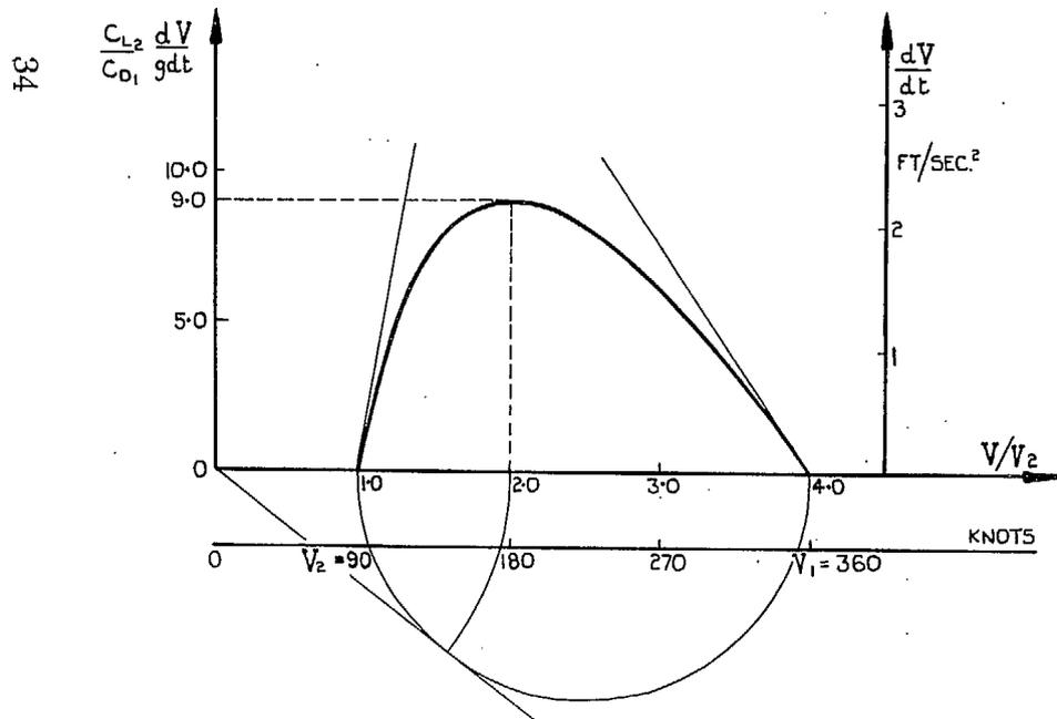
FIG. 4. Acceleration versus speed, at constant height.
