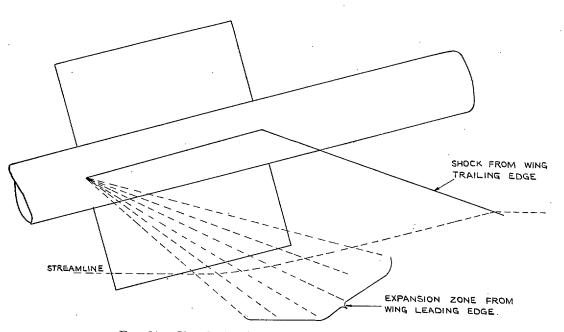
FIG. 21. Sketch showing method of tracing streamline.
