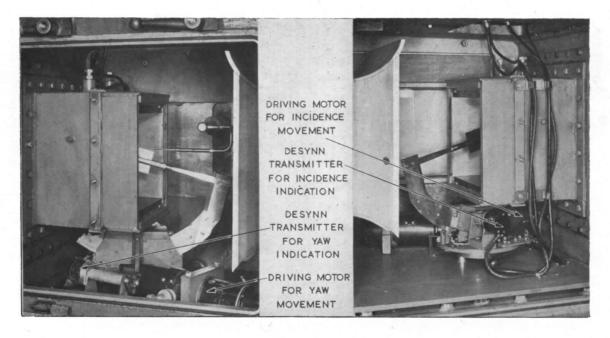
FIG. 2. Model installation in No. 8 (10 in.  $\times$  9 in.) Supersonic Tunnel.
