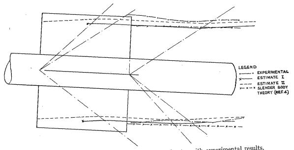
FIG. 23. Vortex-core paths—comparison of estimates with experimental results. Incidence = 20 deg. yaw = -5 deg.
