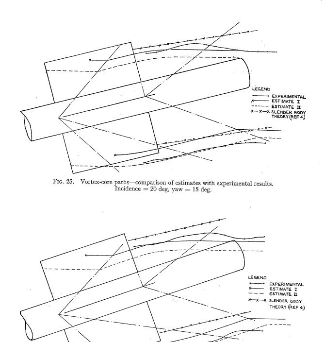
FIG. 26. Vortex-core paths—comparison of estimates with experimental results. Incidence = 20 deg, yaw = 20 deg.
