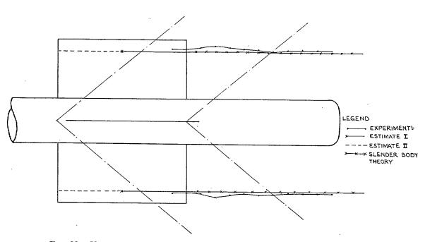
FIG. 22. Vortex-core paths—comparison of estimates with experimental results. Incidence = 20 deg, yaw = 0 deg.
