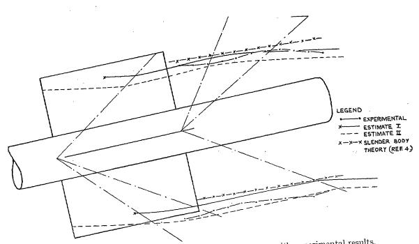
FIG. 24. Vortex-core paths—comparison of estimates with experimental results. Incidence = 20 deg, yaw = 10 deg.
