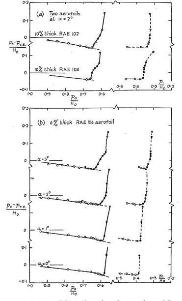
FIG. 18. Effect of section shape and aerofoil incidence on the variation of trailing-edge pressure (Filled symbols denote the presence of separation on the upper surface).
