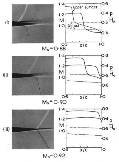
FIG. 24. Sketches to illustrate the changes in the flow on the two surfaces of an aerofoil relative to one another once the lower-surface shock has reached the trailing edge.
