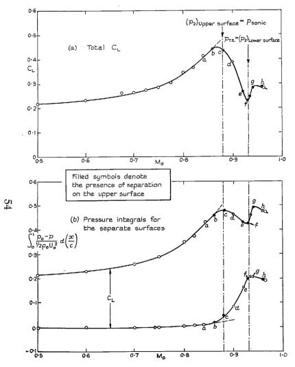
FIG. 34. Observations for a 6 per cent thick RAE 104 aerofoil at 2-deg incidence; variation with free-stream Mach number of the total  $C_L$  and of the contributions from the separate surfaces (See also Figs. 30 to 33).
