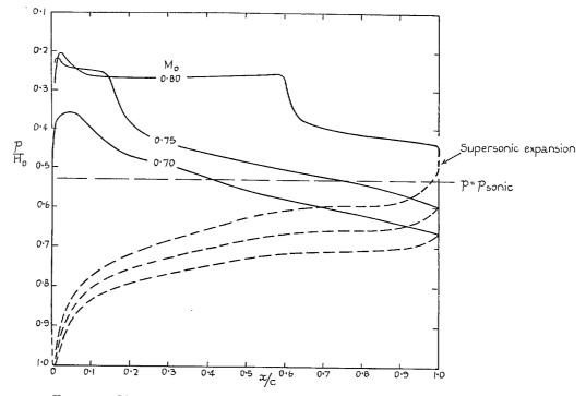
FIG. 27. Observed pressure distributions showing the changes in the flow on the two surfaces of an aerofoil relative to one another when a supersonic expansion occurs at the trailing edge on the lower surface (6 per cent thick aerofoil at 8-deg incidence) (See sketches in Fig. 26).
