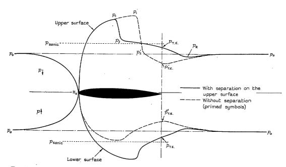
FIG. 4. Sketch of pressure distributions over the surfaces of an aerofoil and along the wake, with and without separation on the upper surface.
