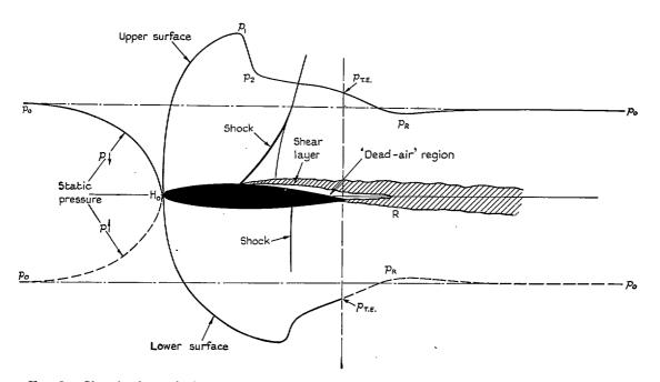
FIG. 3. Sketch of certain features of the flow about an aerofoil and along its wake in the presence of shock-induced separation on the upper surface.
