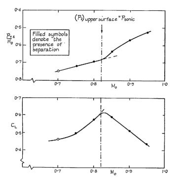
FIG. 39. Observations for a 6 per cent thick RAE 104 aerofoil at 3.7-deg incidence; variation with free-stream Mach number of  $C_{z}$  and  $p_{\text{T.E}}$ (See also Figs. 35 to 38).
