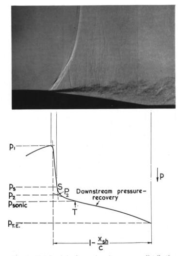
FIG. 6. Details of the flow and surface-pressure distribution near and downstream of separation; definition of certain pressures.
