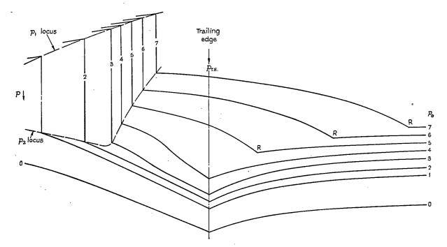
FIG. 14. Idealized sketches of the distributions of pressure from a point just upstream of the uppersurface shock, along the surface and wake to successive values of the free-stream static pressure.
