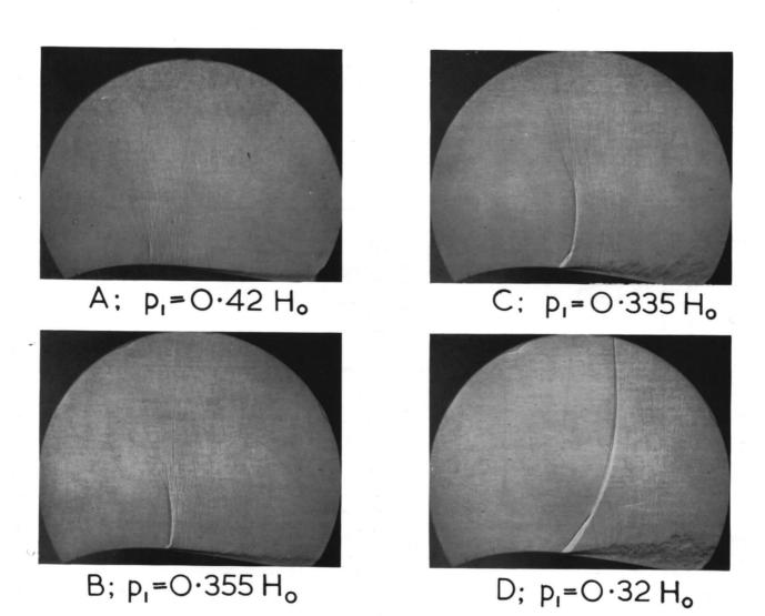
FIG. 11. Photographs showing the development of the separated flow (8 per cent thick half-aerofoil) (See also Fig. 10).
