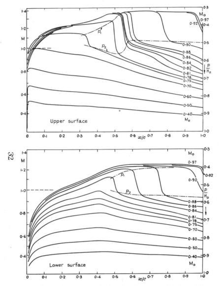
FIG. 1. Surface pressure distributions for a symmetrical aerofoil at a fixed positive incidence (10 per cent thick RAE 102 section at 2-deg incidence).
