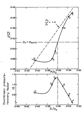
FIG. 37. Observations for a 6 per cent thick RAE 104 aerofoil at 3.7-deg incidence; quantities derived from the upper-surface pressures (See also Figs. 35, 36, 38 and 39) (Filled symbols denote the presence of separation).
