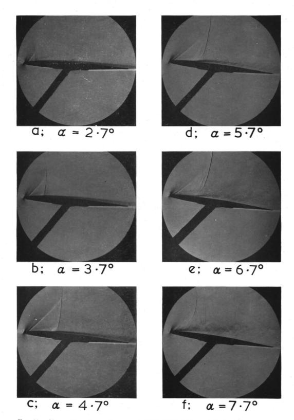
FIG. 41. Observations for a 6 per cent thick RAE 104 aerofoil through a range of incidence;  $M_0 = 0.75$ ; flow photographs (See also Figs. 40, 42 and 43).
