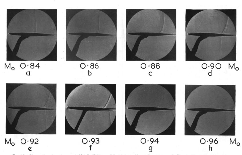
FIG. 31. Observations for a 6 per cent thick RAE 104 aerofoil at 2-deg incidence; flow photographs (See also Figs. 30 and 32 to 34).
