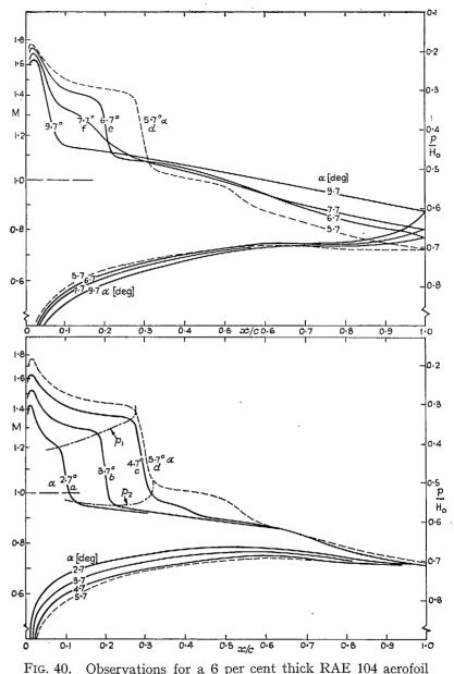
FIG. 40. Observations for a 6 per cent thick RAE 104 aerofoil through a range of incidence;  $M_0 = 0.75$ ; surface-pressure distributions (See also Figs. 41 to 43).
