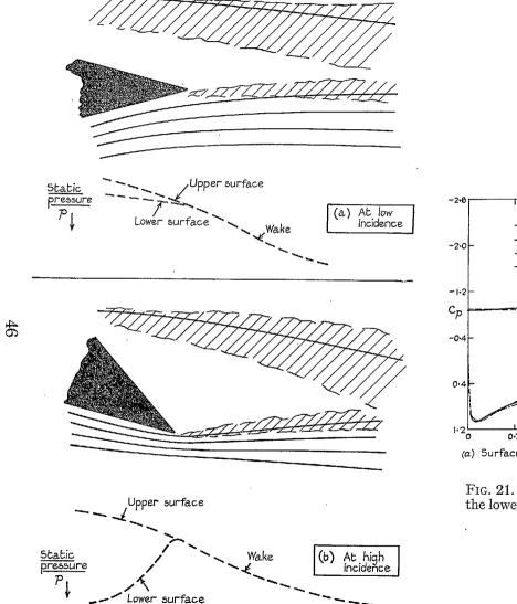
Fig. 20. Sketches to illustrate the influence of the uppersurface separation on the flow near the trailing edge on the lower surface; low and high incidence.
