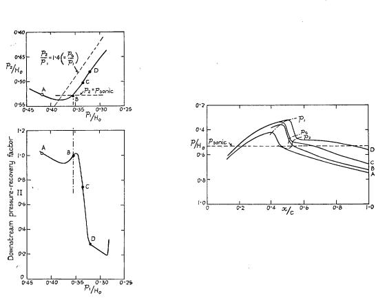
FIG. 10. Surface-pressure distributions, and quantities derived therefrom, at stages in the development of the separated flow (8 per cent thick half-aerofoil) (See Fig. 11 for corresponding flow photographs).
