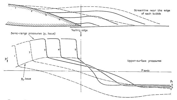
FIG. 28. Sketches to illustrate probable successive stages in the collapse of the separation 'bubble' as the upper-surface shock approaches the trailing edge.
