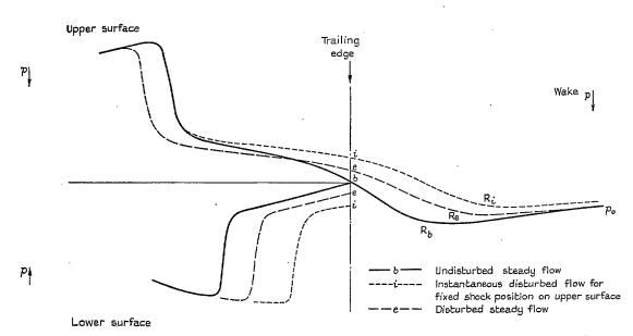
FIG. 16. Sketch of pressure distributions over the rear of an aerofoil and along the wake to illustrate the effect of a hypothetical disturbance to the separated flow near the foot of the shock on the upper surface.
