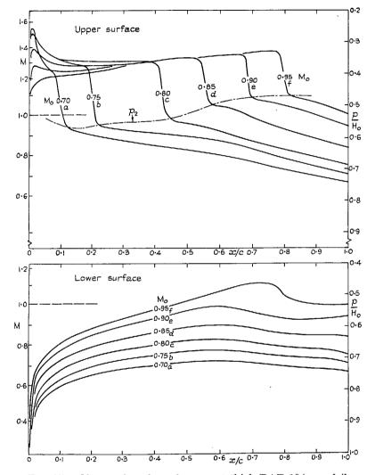
FIG. 35. Observations for a 6 per cent thick RAE 104 aerofoil at 3.7-deg incidence; surface-pressure distributions (See also Figs. 36 to 39).
