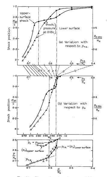
FIG. 33. Observations for a 6 per cent thick RAE 104 aerofoil at 2-deg incidence; variation of a flow parameter (shock position or pressure at a fixed point) for each surface (See also Figs. 30, 31, 32 and 34).
