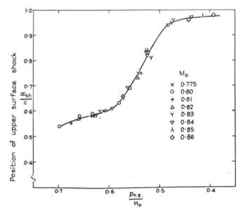
FIG. 5. Variation of upper-surface shock position with trailing-edge pressure, as adjusted by changing the height and position of a small strip on the lower surface.
