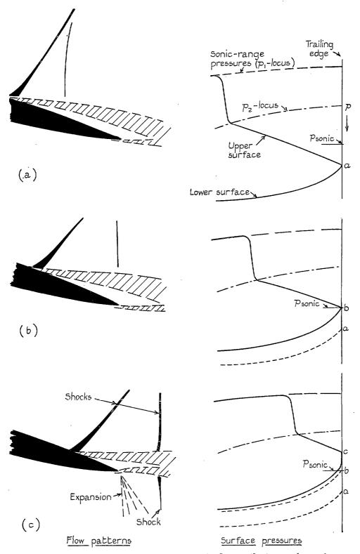
FIG. 26. Sketches to illustrate the changes in the flow on the two surfaces of an aerofoil relative to one another once a supersonic expansion can occur at the trailing edge on the lower surface.
