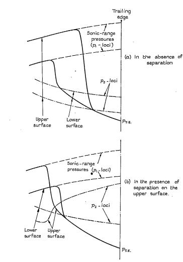
FIG. 22. Sketches of surface-pressure distributions to show relative shock positions for an aerofoil at a fairly low incidence and a Mach number close to unity.
