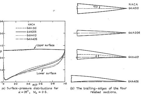
FIG. 21. The influence of trailing-edge angle and camber on the pressures over the lower surface in the presence of severe separation on the upper surface (results for four related NACA sections; Ref. 23).
