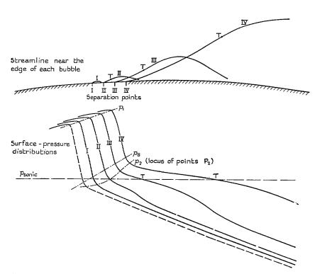
FIG. 9. Sketches to illustrate successive stages in the development of the separation 'bubble' for a prescribed variation of  $p_1$ .
