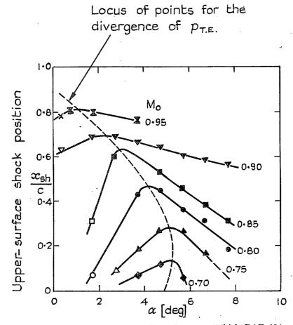
FIG. 44. Observations for a 6 per cent thick RAE 104 aerofoil through a range of incidence; upper-surface shock positions for several different constant Mach numbers (Filled symbols denote the presence of separation).
