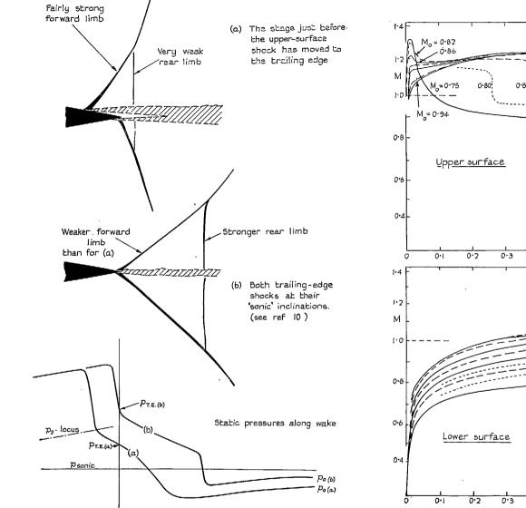
FIG. 29. Movement of the shocks into their 'sonic' positions and inclinations.
