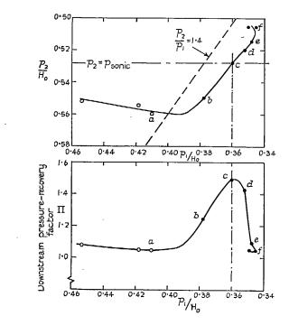
FIG. 32. Observations for a 6 per cent thick RAE 104 aerofoil at 2-deg incidence; quantities derived from the upper-surface pressures (See also Figs. 30, 31, 33 and 34). (Filled symbols denote the presence of separation.)
