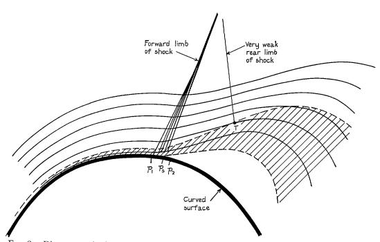
FIG. 8. Diagrammatic sketch of streamlines and boundary flow near separation on a curved surface (curvature greatly exaggerated). T is the approximate position at which the velocity along the streamline has fallen to the sonic value.
