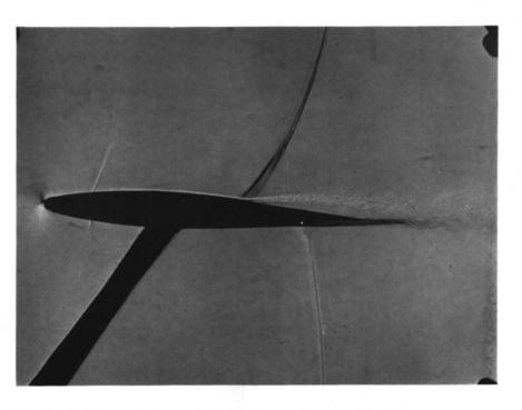
FIG. 2. Schlieren photograph of the flow past an aerofoil with severe separation at the foot of the upper-surface shock; 10 per cent RAE 102 section at 2-deg incidence ( $M_0 = 0.88$ ).
