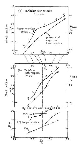
FIG. 38. Observations for a 6 per cent thick RAE 104 aerofoil at  $3 \cdot 7$ -deg incidence; variation of a flow parameter (shock position and pressure at a fixed point) for each surface (*See* also Figs. 35, 36, 37 and 40).
