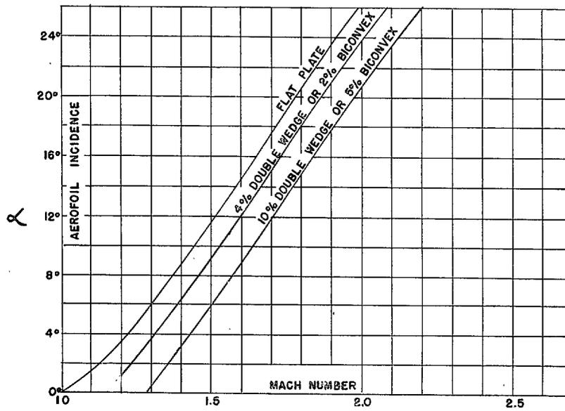
FIG. 6. Limiting Incidence for Exact Theory to Apply.
