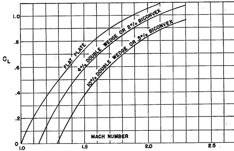
FIG. 8. Limiting  $C_L$  for Exact Wing Theory to Apply.
