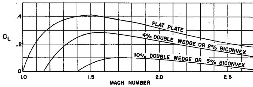
FIG. 7. Limiting  $C_L$  for Busemann's Second-order Theory to be .1 per cent in Error on Pressure.
