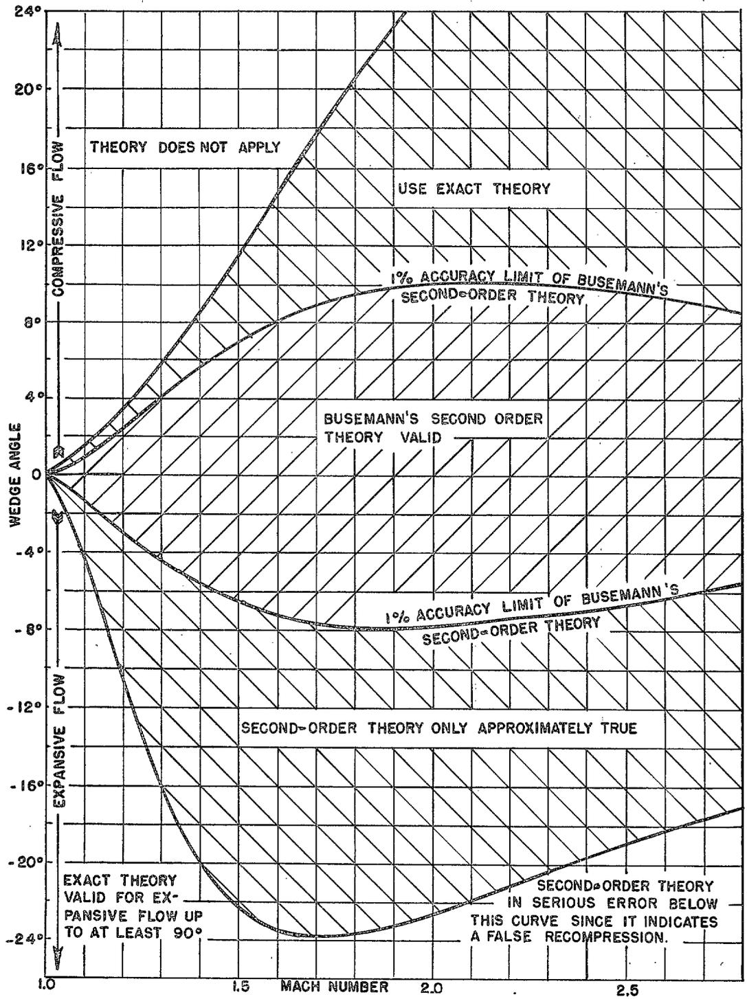
FIG. 3. Limiting Wedge Angles as a Function of Mach Number.
