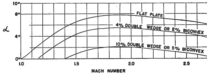
FIG. 5. Limiting Incidence for Busemann's Second-order Theory to be 1 per cent in Error on Pressure.
