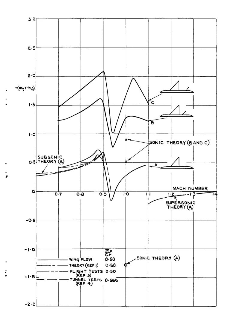
FIG.5.COMPARISON OF  $-(m_{2} + m_{di})$ FOR THE THREE. CONFIGURATIONS, A, B AND C.
