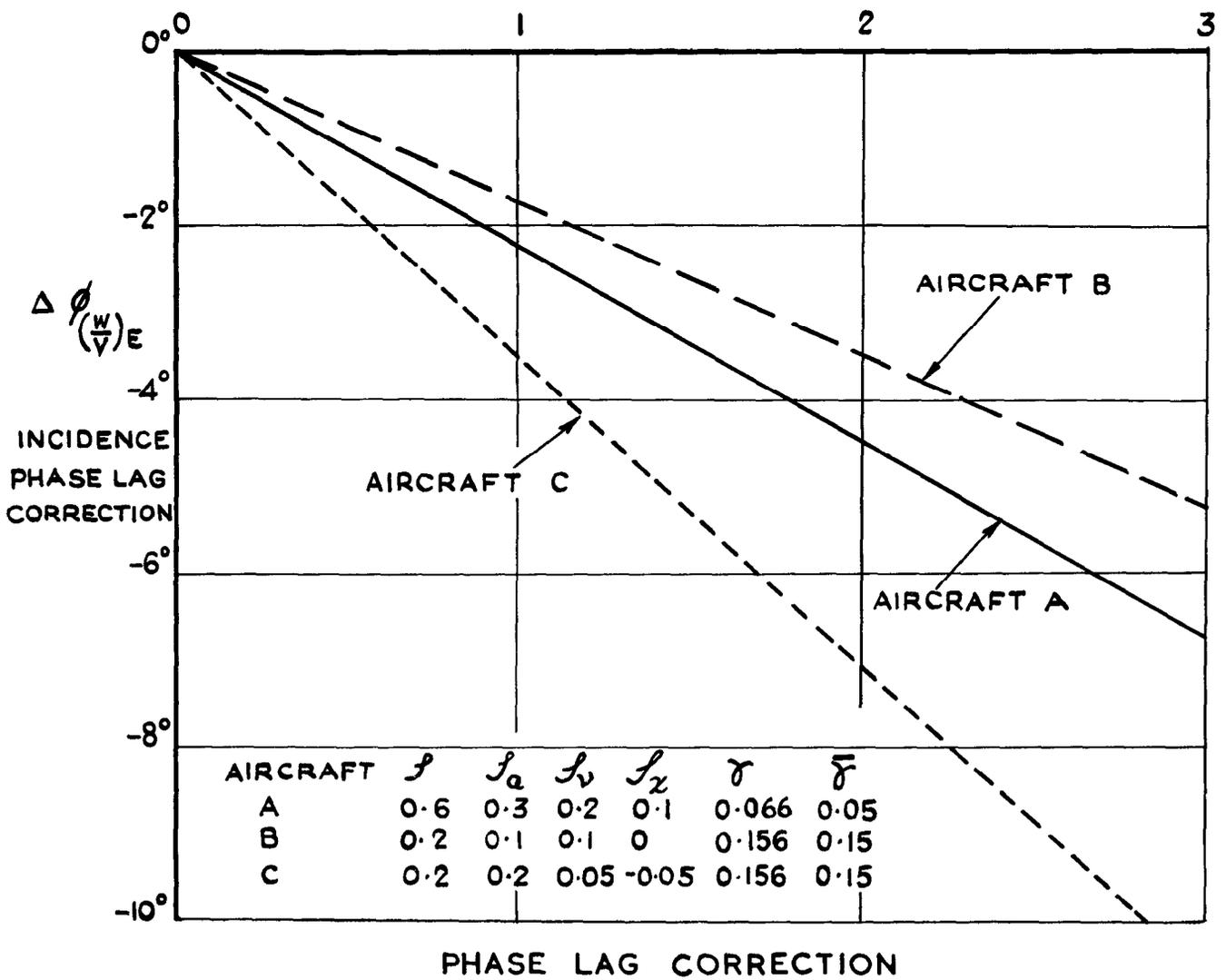
FIG.5 AN EXAMPLE OF THE EFFECT OF ELEVATOR LIFT ON THE FREQUENCY RESPONSE OF INCIDENCE TO ELEVATOR
