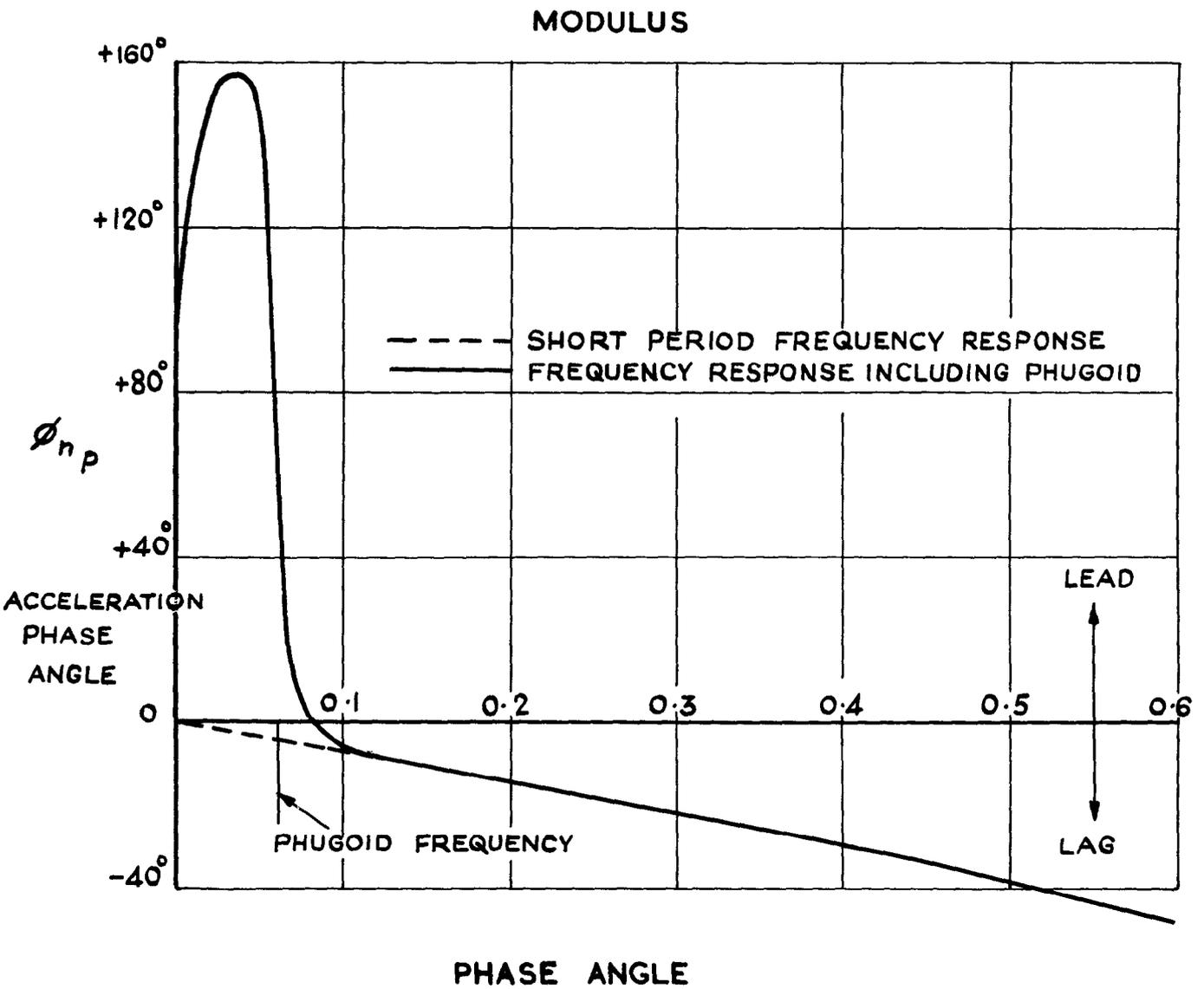
FIG.10. AN EXAMPLE PHUGOID FREQUENCY RESPONSE CURVES FOR NORMAL ACCELERATION
