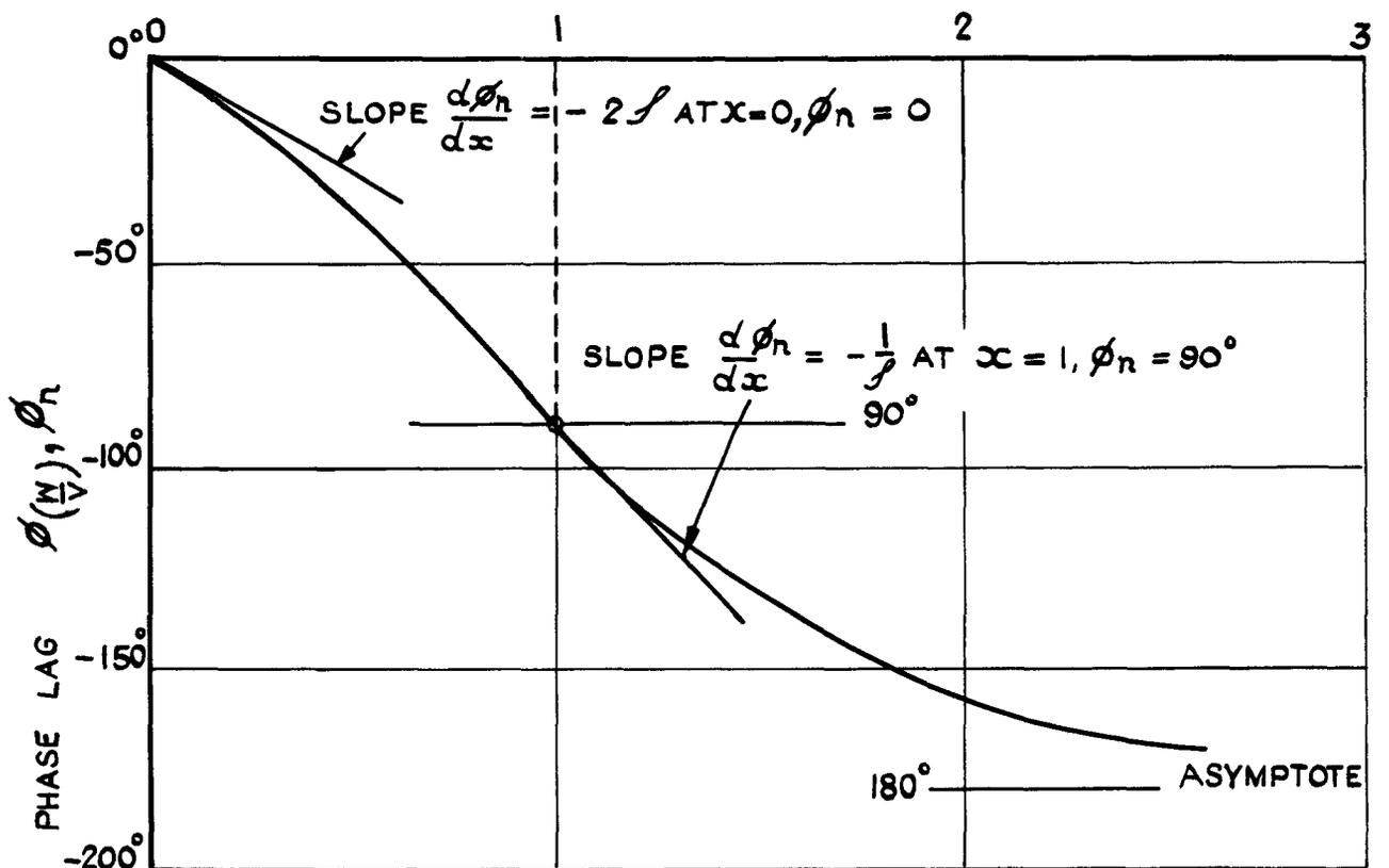
FIG. I. THE CHARACTERISTICS OF THE NON-DIMENSIONAL SHORT PERIOD FREQUENCY RESPONSE OF INCIDENCE AND NORMAL ACCELERATION
