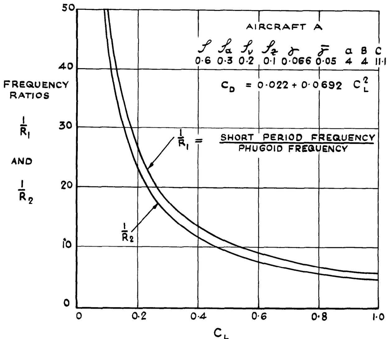
FIG.15 RATIO OF SHORT PERIOD FREQUENCY TO PHUGOID FREQUENCY,  $\frac{1}{R_1}$  AND THE RATIO  $\frac{1}{R_2}$  FOR DIFFERENT LIFT COEFFICIENTS (AIRCRAFT A)
