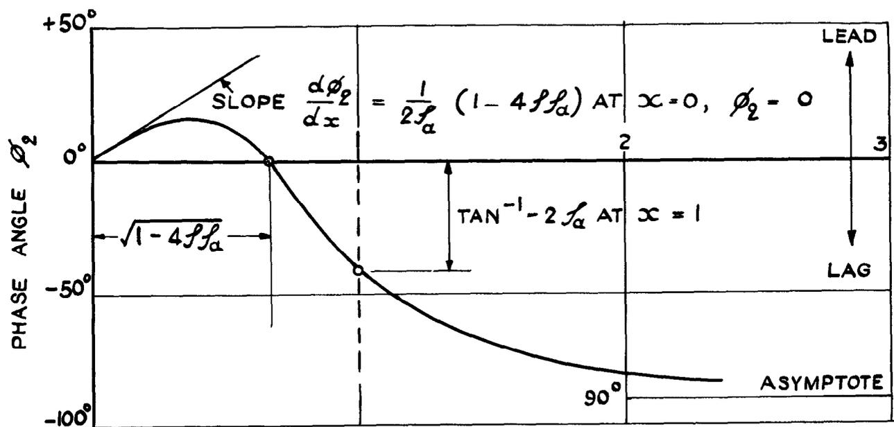
FIG.2. THE CHARACTERISTICS OF THE NON-DIMENSIONAL SHORT PERIOD FREQUENCY RESPONSE OF RATE OF PITCH
