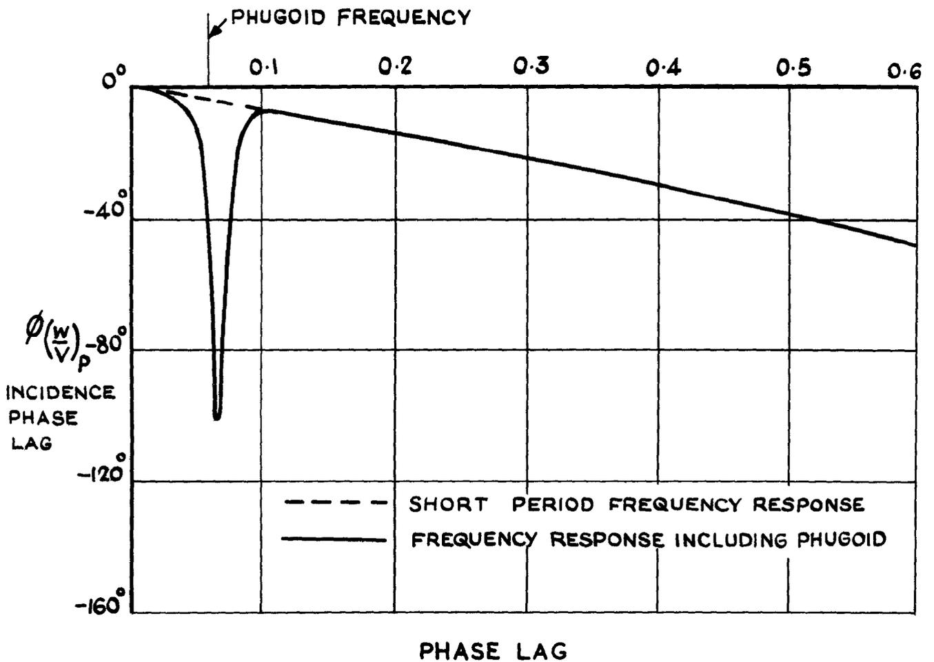
**FIG.9. AN EXAMPLE OF PHUGOID FREQUENCY RESPONSE CURVES FOR INCIDENCE**
