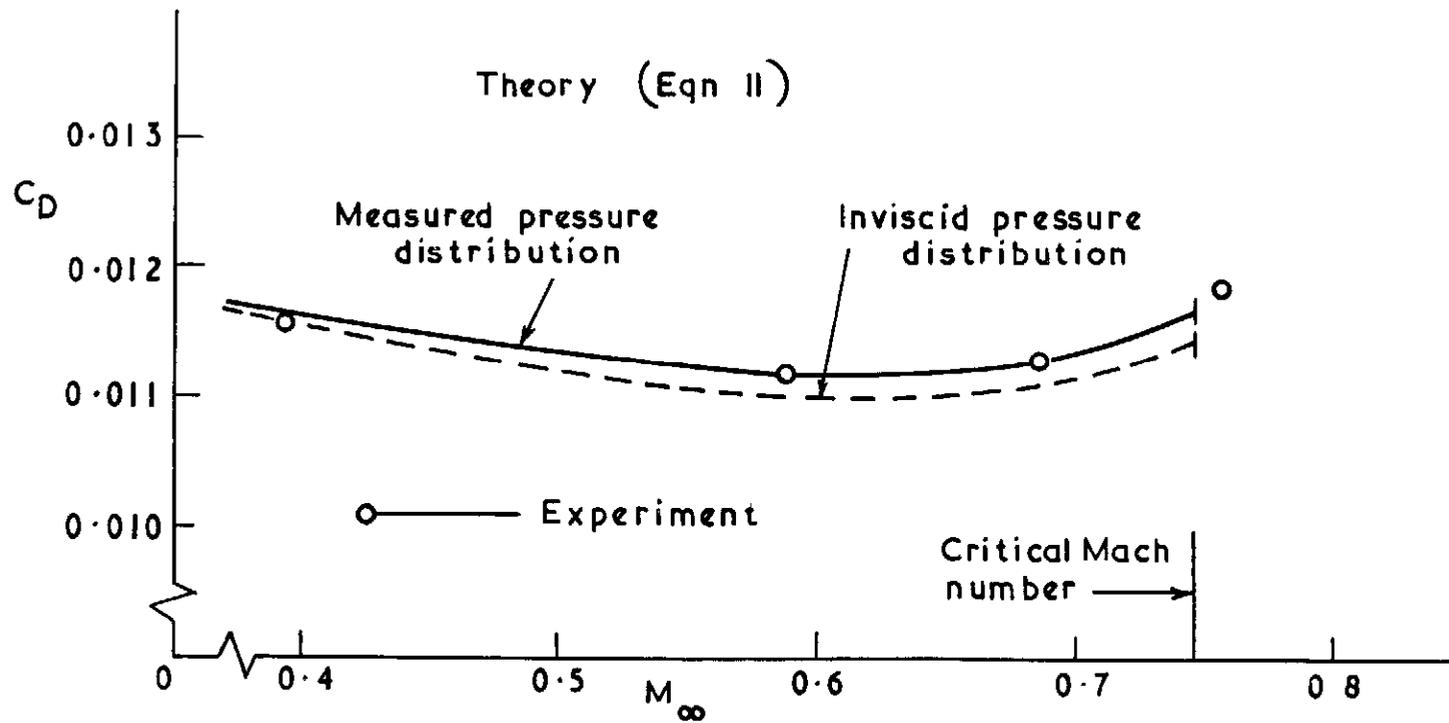
Effect on predicted  $C_D$  of using measured pressure distribution
